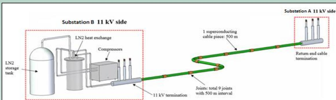
Illustration of a Superconducting cable system transferring power from Substation B to Substation A.
