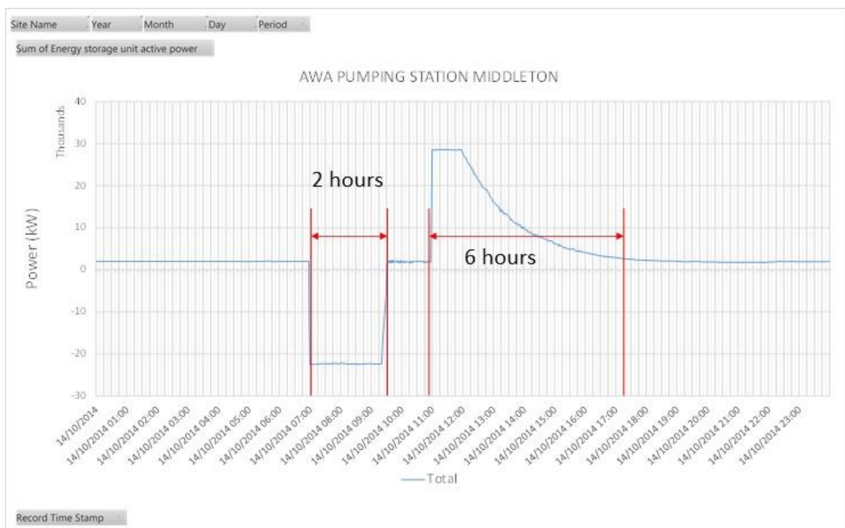
Figure 8: Illustration of charge and discharge periods for available battery capacity
