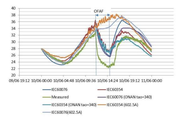
Figure 36: Top-oil temperature comparison, T1, OFAF trial 12.00 – 15.00, 10<sup>th</sup> Jun 2015
