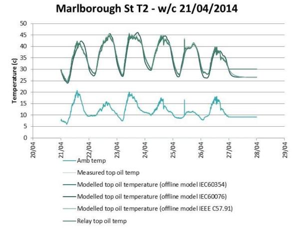
Figure 42 : Top-oil temperature modelling results with different models compared to measured and relay values (T2, w/c 21/04/2014).
