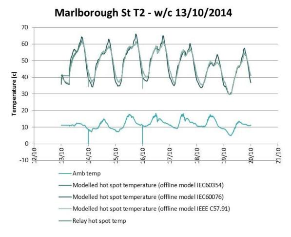
Figure 68 : Hot-spot temperature modelling results with different models compared to relay values (T2, w/c 13/10/2014).
