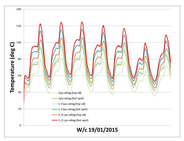
Figure 22 : of hotspot (and top oil) temperatures associated with the modelled load current (peaking at 19MVA equivalent), with the experienced ambient air temperatures)
