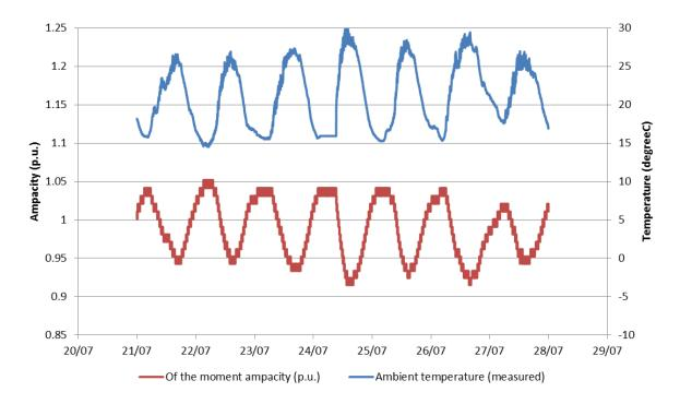
Figure 76: Of-the-moment ampacity (load factor) (ambient temperature w/c 21/07/2014) – High summer.
