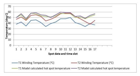
Figure 14: Hot spot temperature modelling results compared to measured WTI values
