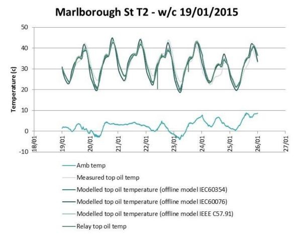
Figure 50 : Top-oil temperature modelling results with different models compared to measured and relay values (T2, w/c 19/01/2015).
