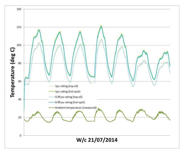
Figure 21 : of hotspot (and top oil) temperatures associated with the modelled load current (peaking at 19MVA equivalent), with the experienced ambient air temperatures)
