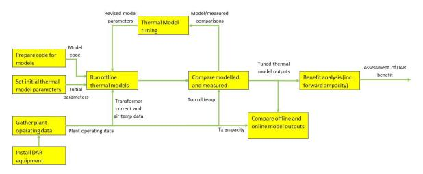
Figure 2: overall process approach to the technique trial
