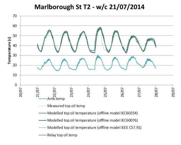
Figure 46 : Top-oil temperature modelling results with different models compared to measured and relay values (T2, w/c 21/07/2014).
