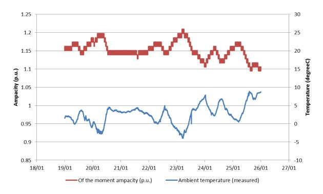
Figure 78: Of-the-moment ampacity (load factor) (ambient temperature w/c 19/01/2015) - Winter.
