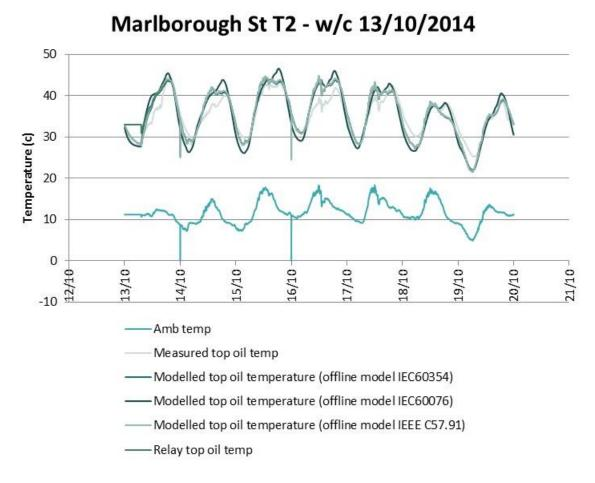
Figure 48 : Top-oil temperature modelling results with different models compared to measured and relay values (T2, w/c 13/10/2014)
