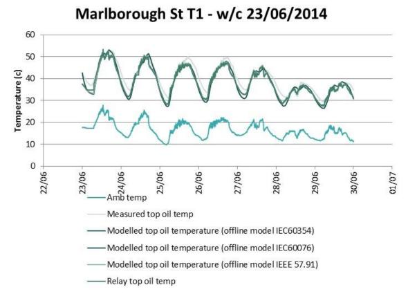
Figure 43 : Top-oil temperature modelling results with different models compared to measured and relay values (T1, w/c 23/06/2014).
