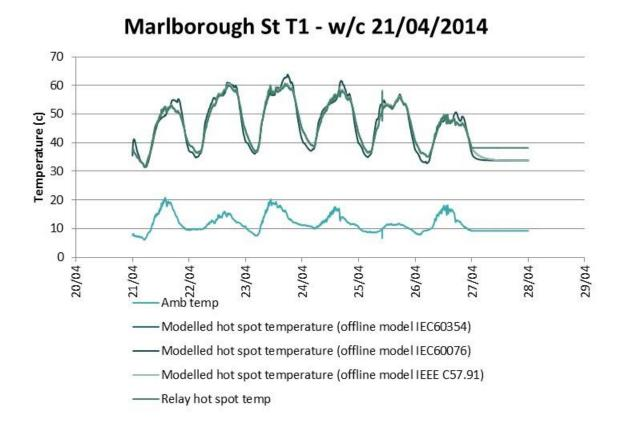
Figure 61 : Hot-spot temperature modelling results with different models compared to relay values (T1, w/c 21/04/2014).
