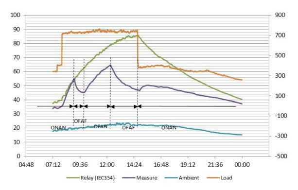
Figure 16: Top-oil temperature comparison, T1, ONAN, 9<sup>th</sup> Jul 2014
