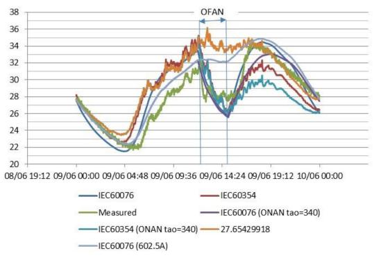
Figure 35: Top-oil temperature comparison, T1, OFAN trial 12.00 – 15.00, 9<sup>th</sup> Jun 2015
