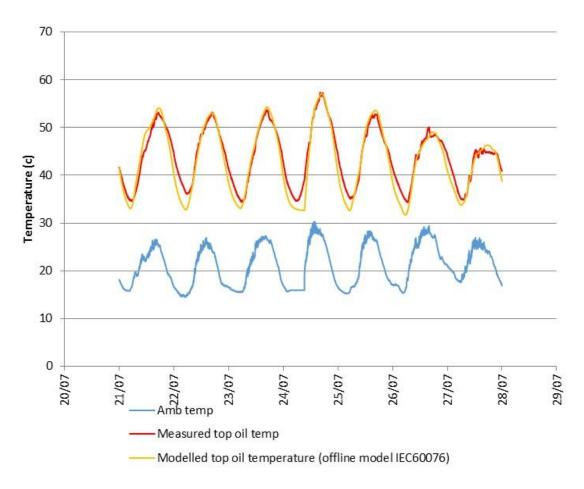
Figure 12: Top-oil temperature modelling results for Marlborough St T1 - w/c 21/07/2014
