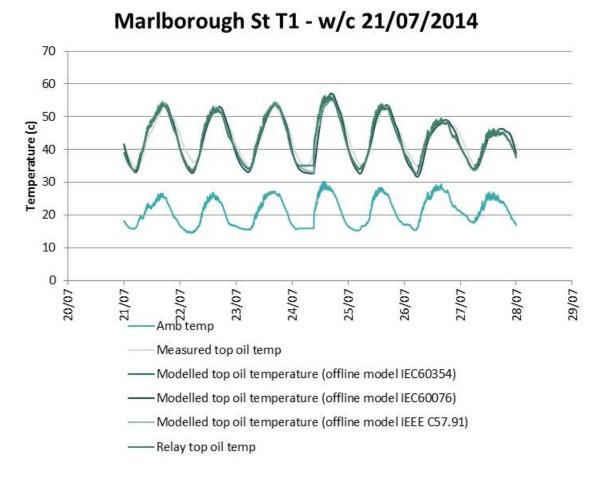
Figure 45 : Top-oil temperature modelling results with different models compared to measured and relay values (T1, w/c 21/07/2014).
