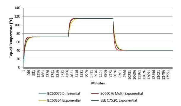
Figure 32: Top oil temperature calculation with different models (long-term step loading)
