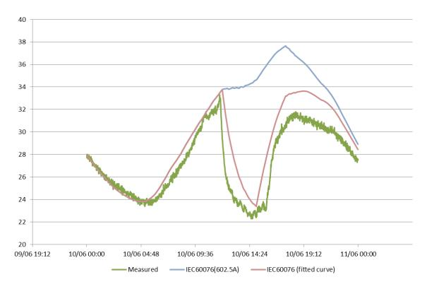
Figure 39: Top-oil temperature comparison with curve fitting results, T1, OFAF trial 12.00 – 15.00, 10<sup>th</sup> Jun 2015
