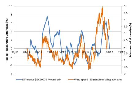
Figure 72: Comparisons between model-calculated and measured oil temperature values with wind speed (w/c 01/12/2014)
