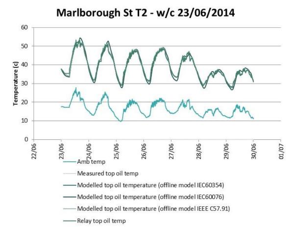
Figure 44 : Top-oil temperature modelling results with different models compared to measured and relay values (T2, w/c 23/06/2014).
