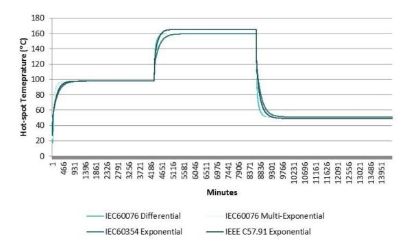
Figure 33: Hot-spot temperature calculation with different models (long-term step loading)
