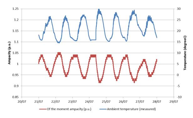
Figure 19 : Dynamic rating and ambient air temperature for w/c 21/07/2014 – High summer.
