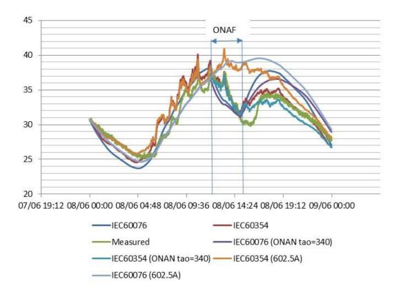
Figure 34: Top-oil temperature comparison, T1, ONAF trial 12.00 – 15.00, 8<sup>th</sup> Jun 2015
