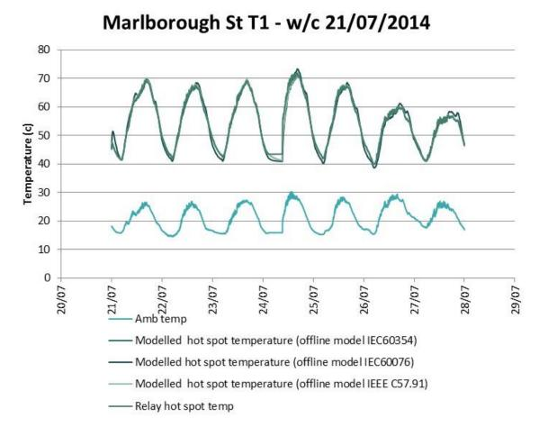
Figure 65 : Hot-spot temperature modelling results with different models compared to relay values (T1, w/c 21/07/2014).
