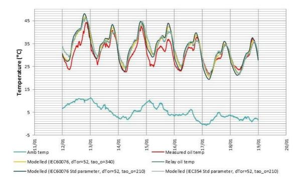
Figure 8: Modelling results with different models and model parameter values (T1, w/c 12/01/2015)
