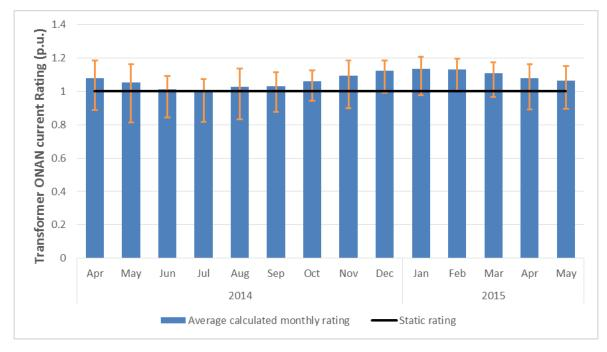
Figure 20 : Primary transformer T1 monthly dynamic rating limits under ONAN cooling for unit loss-of-life operation (98°C limit)
