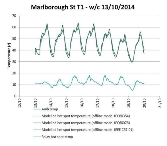
Figure 67 : Hot-spot temperature modelling results with different models compared to relay values (T1, w/c 13/10/2014).
