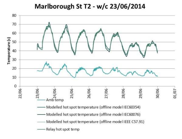
Figure 64 : Hot-spot temperature modelling results with different models compared to relay values (T2, w/c 23/06/2014).
