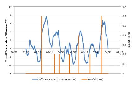
Figure 73: Comparisons between model-calculated and measured oil temperature values with precipitation (w/c 01/12/2014)
