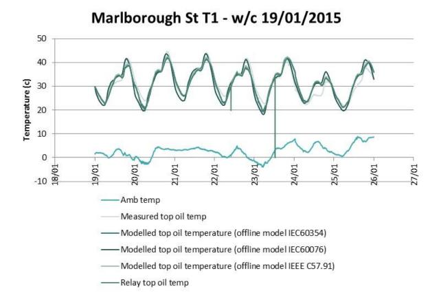
Figure 49 : Top-oil temperature modelling results with different models compared to measured and relay values (T1, w/c 19/01/2015).
