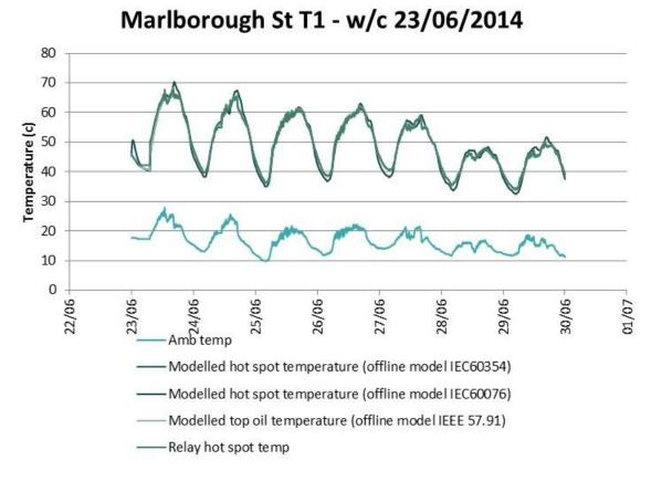
Figure 63 : Hot-spot temperature modelling results with different models compared to relay values (T1, w/c 23/06/2014).
