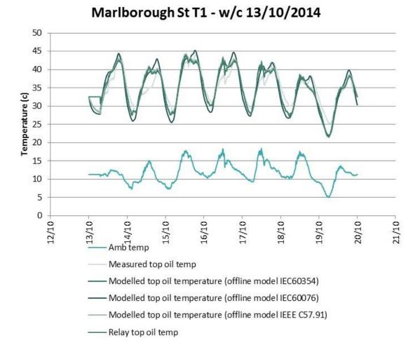
Figure 47 : Top-oil temperature modelling results with different models compared to measured and relay values (T1, w/c 13/10/2014)
