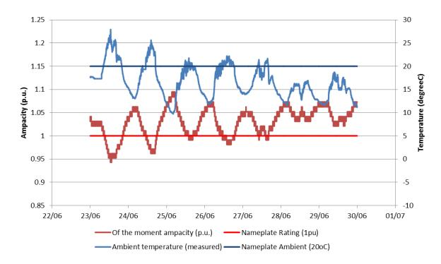
Figure 75: of-the-moment ampacity (load factor) (ambient temperature w/c 23/06/2014) – Summer.
