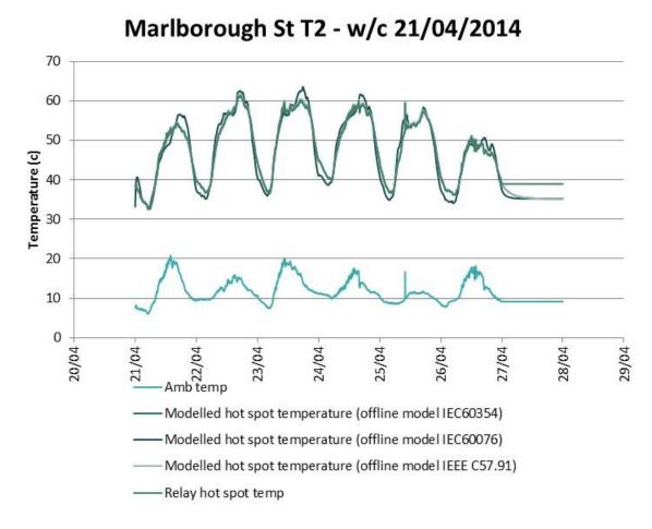
Figure 62 : Hot-spot temperature modelling results with different models compared to relay values (T2, w/c 21/04/2014).
