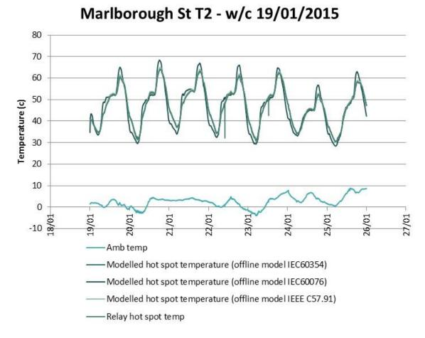
Figure 70 : Hot-spot temperature modelling results with different models compared to relay values (T2, w/c 19/01/2015).
