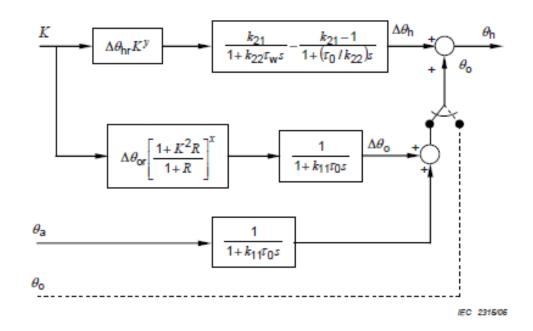
Figure 1: Outline of the IEC 60076 calculation of hot-spot temperature [2]
