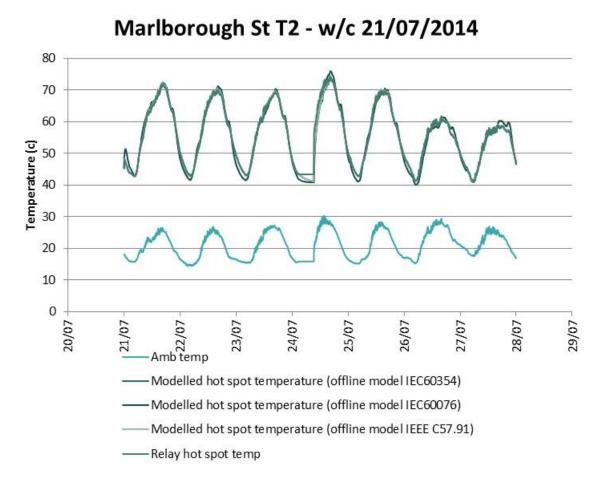
Figure 66 : Hot-spot temperature modelling results with different models compared to relay values (T2, w/c 21/07/2014).
