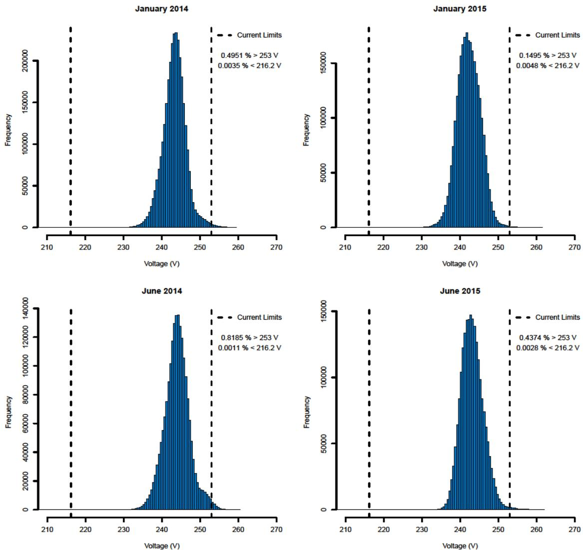
**Figure 7: Substation voltage distributions**
