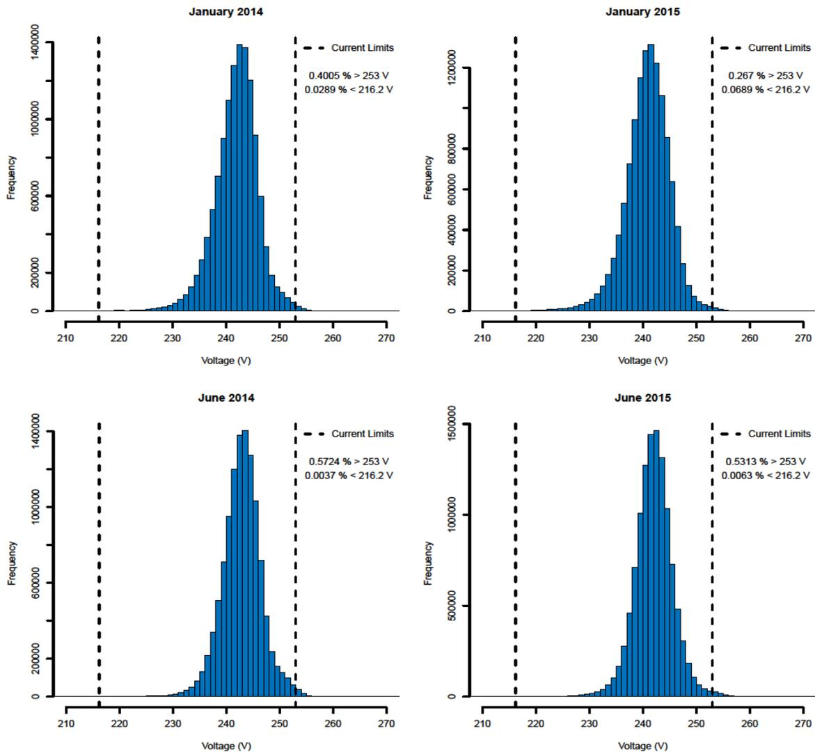
**Figure 8: Feeder end voltage distributions**
