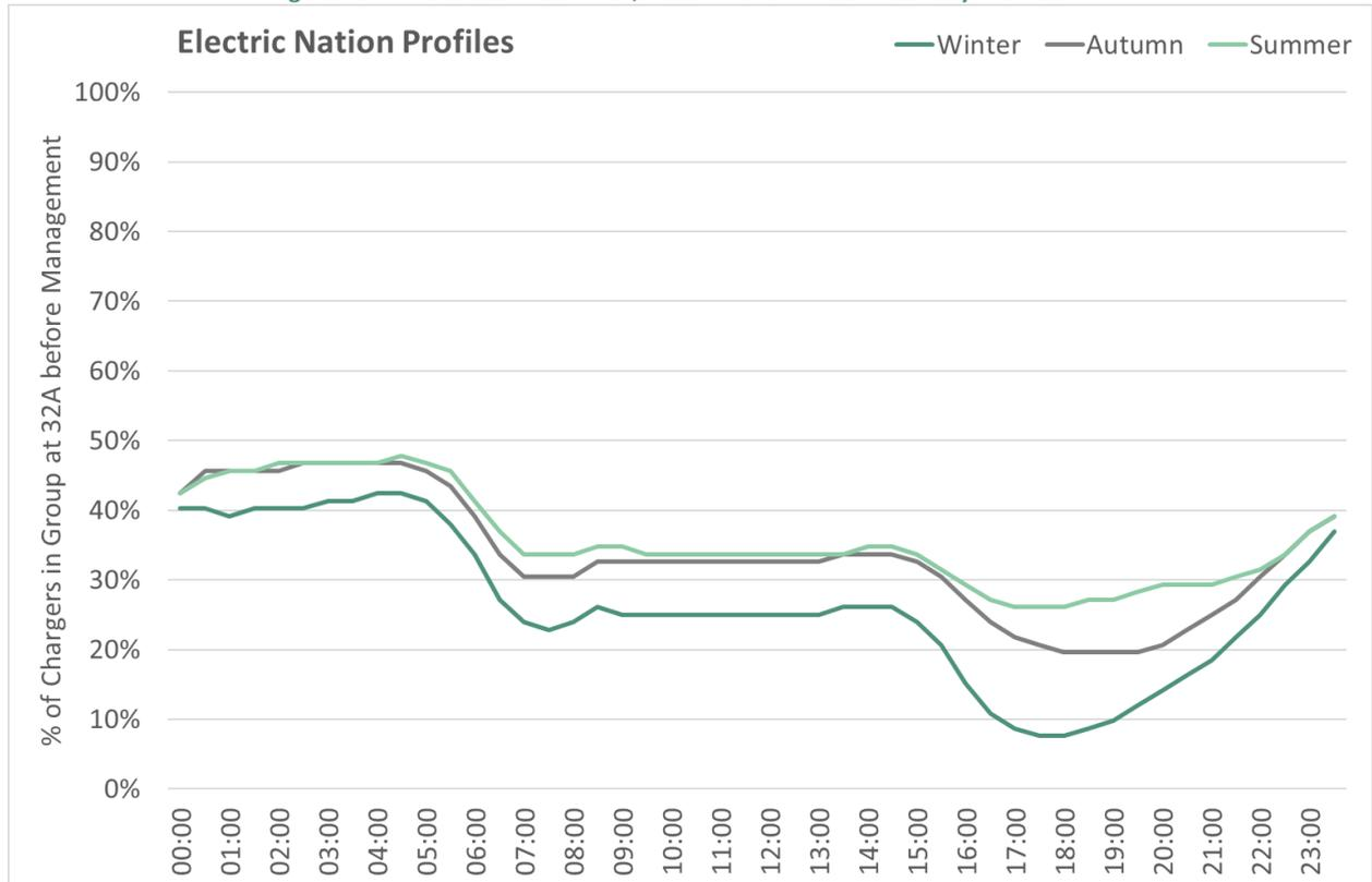
In the autumn example above, on each weekday 19% of the 92 stations in the group can charge at 32A at 19:00. Therefore, if on a given weekday only 15 chargers were being used at this time then no management would occur. Graphs such as the above provide an indication of how restrictive a given profile is but cannot predict whether management will occur on any given day, as this depends on the charging behaviour of each participant.
