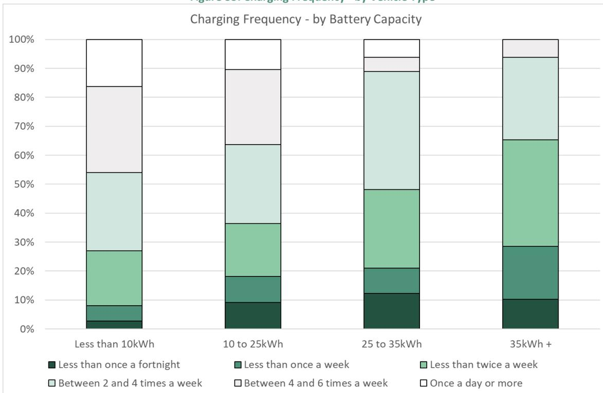
This indicates that the majority of participants charge less than four times a week. As expected, charging every day is more prevalent for participants with smaller batteries and therefore lower ranges (less than 10kWh and 10 to 25kWh).
