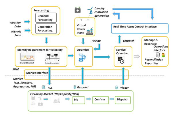
Figure 2: Our vision for a DSO flexibility Solution
