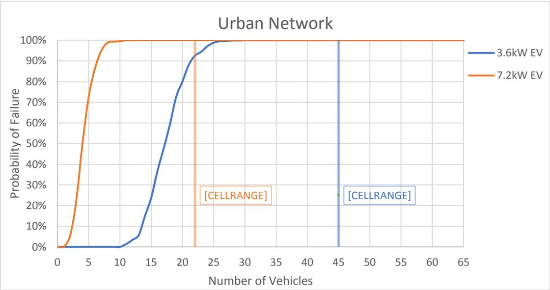
Figure C-4: Urban network with upper quartile EV profile, 0% background harmonic distortion and  $Z_h$  as per equation 2-1
