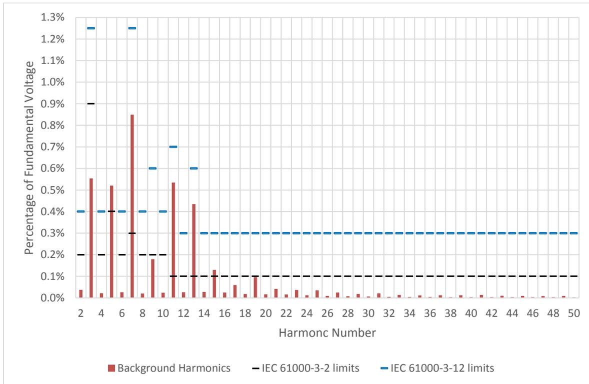
**Figure 3 Average background voltage distortion compares against IEC 61000-3-2 and -12 limits**
