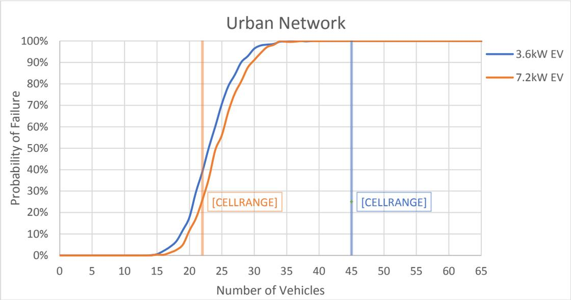
Figure C-3: Urban network with median EV profile, 0% background harmonic distortion and  $Z_h$  as per equation 2-1
