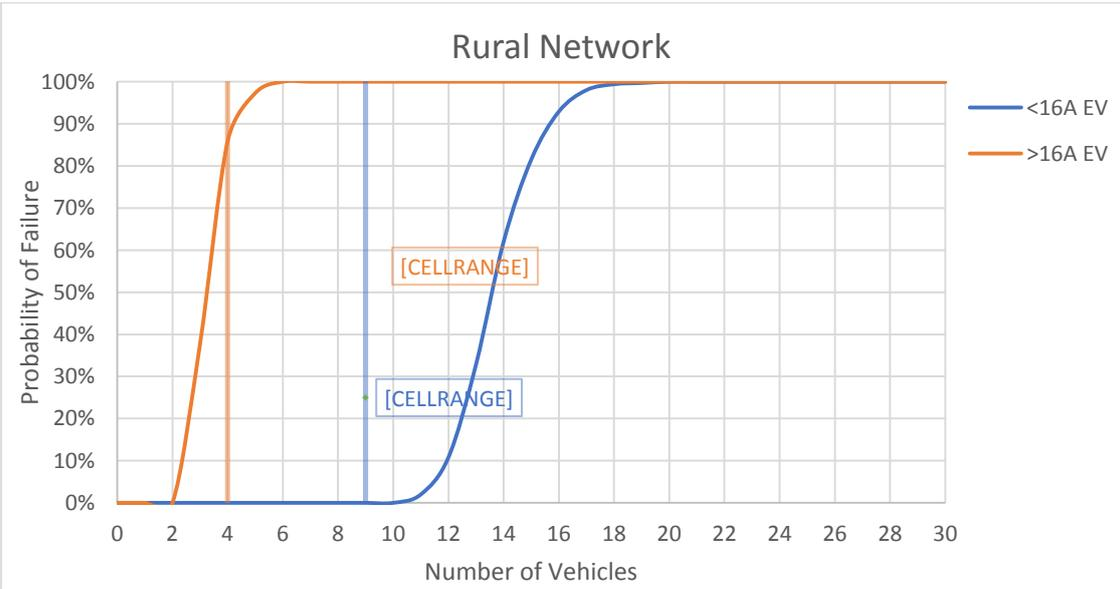
Figure C-12: Rural network with upper quartile EV profile, 0% background harmonic distortion and  $Z_h$  as per equation 2-2
