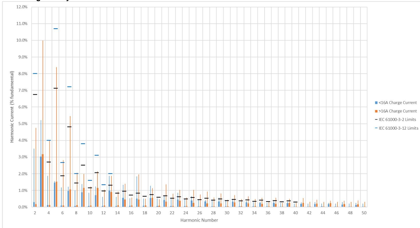
Figure 3-7: Upper quartile typical EV harmonic current for <16 A and >16 A charging currents
