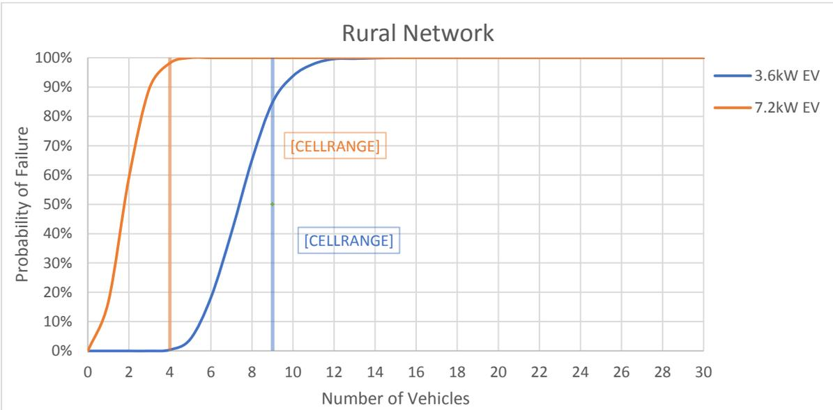
Figure C-6: Rural network with typical upper quartile EV harmonic current, WPD background harmonic distortion and  $Z_h$  calculated as per equation 2-1
