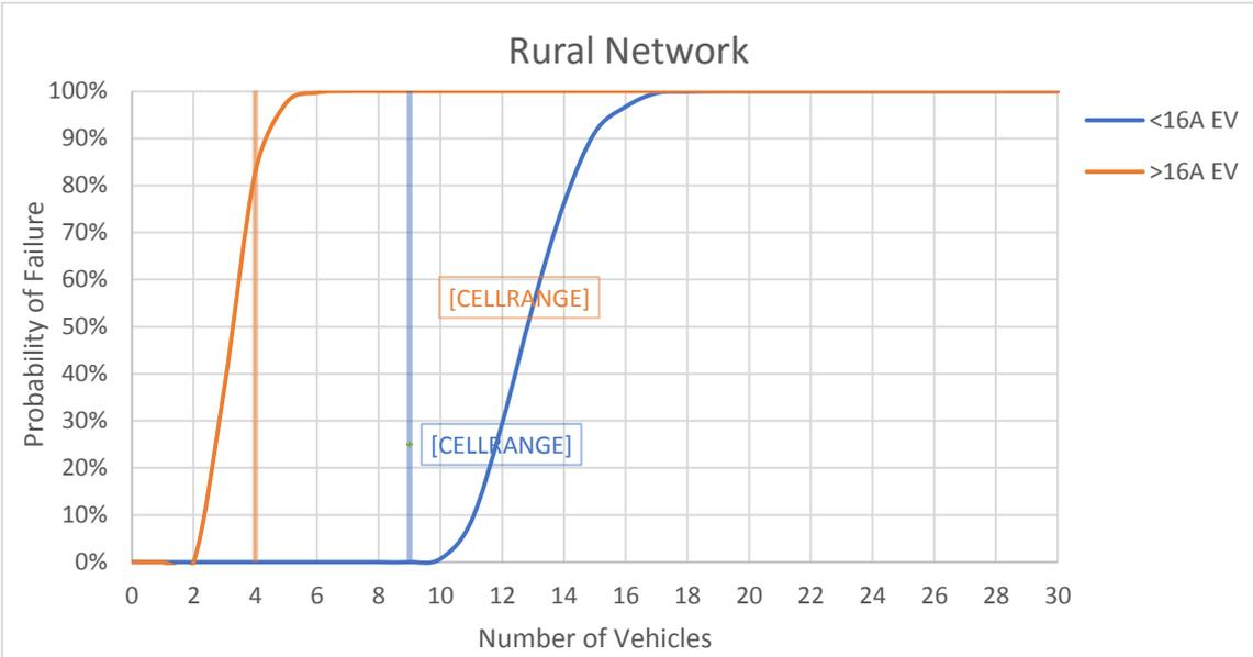
Figure 4-4: Rural network with typical upper quartile EV harmonic current, WPD background harmonic distortion and  $Z_h$  calculated as per equation 2-2
