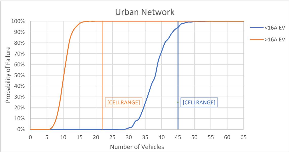
Figure 4-2: Urban network with upper quartile EV profile, WPD background harmonic distortion and  $Z_h$  as per equation 2-2
