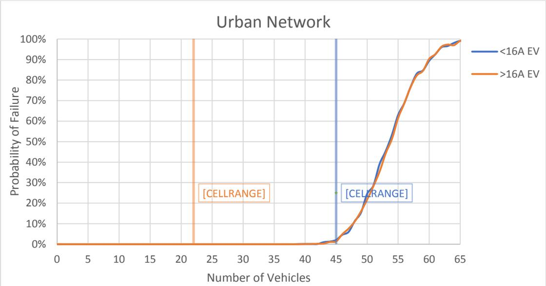
Figure C-9: Urban network with median EV profile, 0% background harmonic distortion and  $Z_h$  as per equation 2-2
