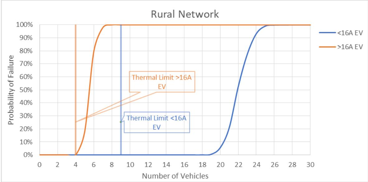
Figure 4-6: Rural network with a maximum source impedance of 0.21+j0.126 Ω with typical upper quartile EV harmonic current, WPD background harmonic distortion and Z<sub>n</sub> calculated as per equation 2-2
