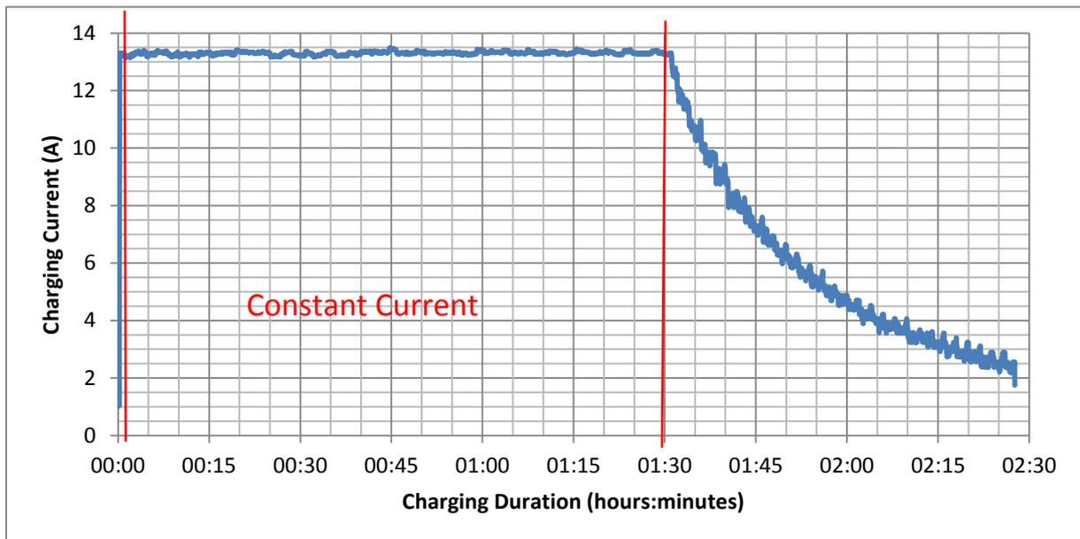
Figure 2: Typical 3.2 kW charging profile with extracted constant current section marked
