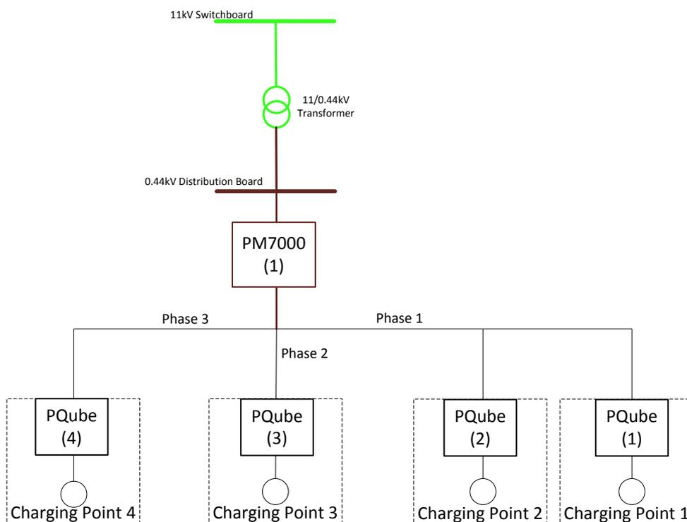
**Figure 1: Vehicle charger and power quality measurement device arrangement**
