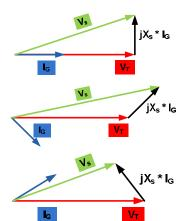
Figure 2: The vector calculation for generator internal voltage when it operates at (from top to bottom) Unity power factor, Lagging power factor, and Leading power factor
