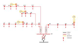
Figure 4: The sample model representing a short and a long feeder
