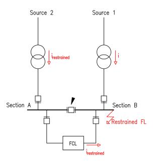
**Figure 1: Typical FCL Installation**
