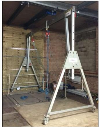
Figure 2-10: Portable lifting frame used to lift the cryostat vessels to the first floor
