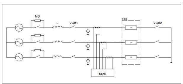
Figure 2-9: Connection diagram showing the KEMA short circuit test set-up for Chester Street FCL
