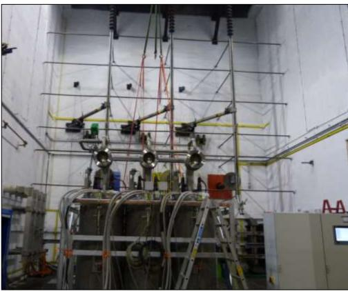
Figure 2-8: Photograph of Bournville FCL during short circuit testing in KEMA lab, Arnhem, Netherlands
