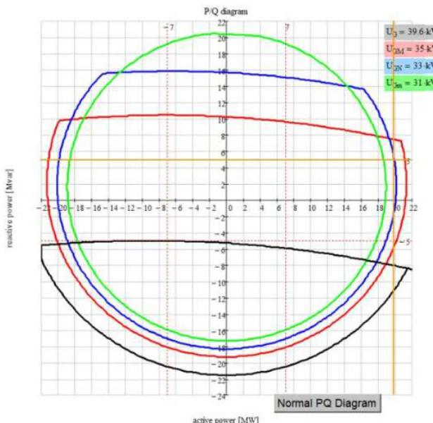
Figure 2-23: FPL1 20MW, 5MVar (@ 34kV)
