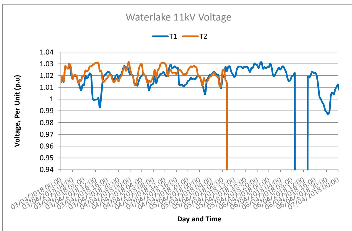
Figure 2-7 Waterlake 11kV Voltage
