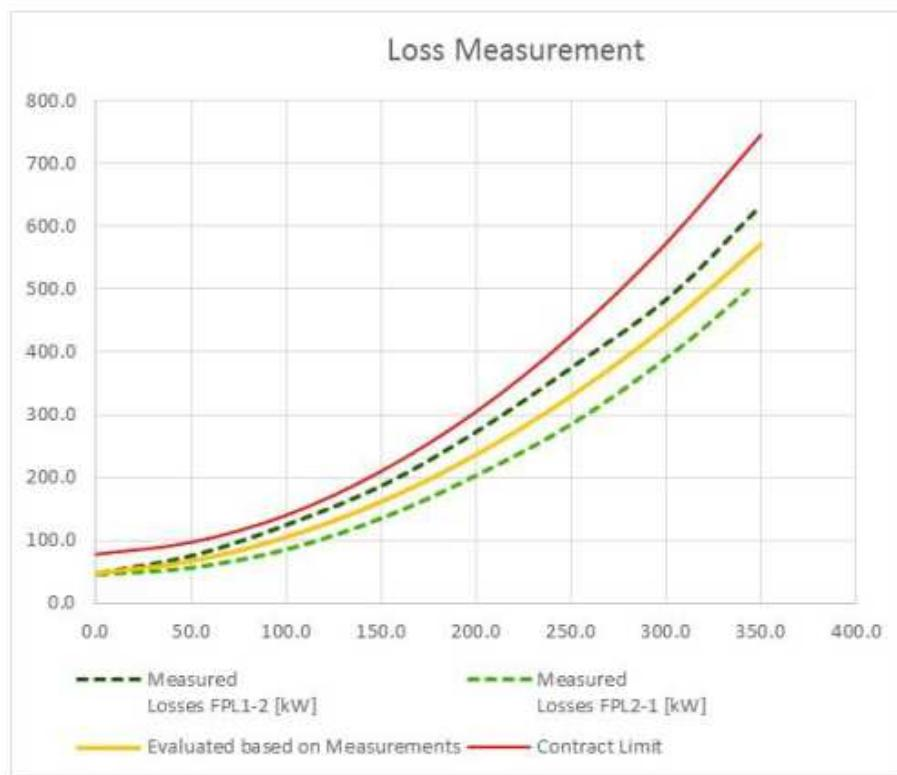
Figure 2-22: FPL Loss Measurement under Test
