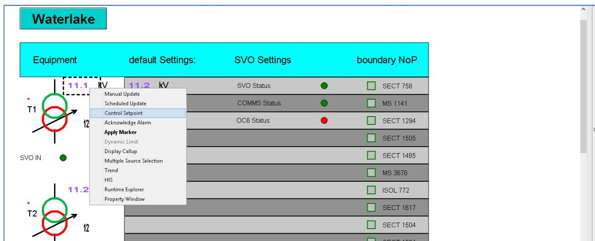
Figure 2-1 Manual Sending of Set Points through SP5
