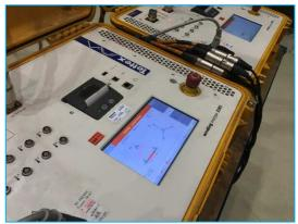
Figure 2-23: Winding resistance test
