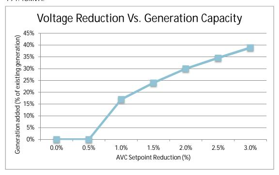
It is estimated that the combination of the EVA and SVO methods (i.e. reduction of the AVC setpoint along with an increase of the allowable voltage limits) would result in at least 10% further increase of the overall capacity release, as compared to the separate implementation of the two methods.
