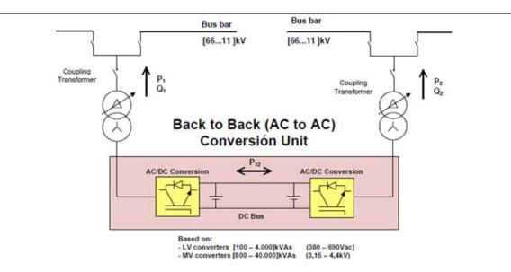
Figure 4 - Flexible Power Link Schematic (Indicative)
