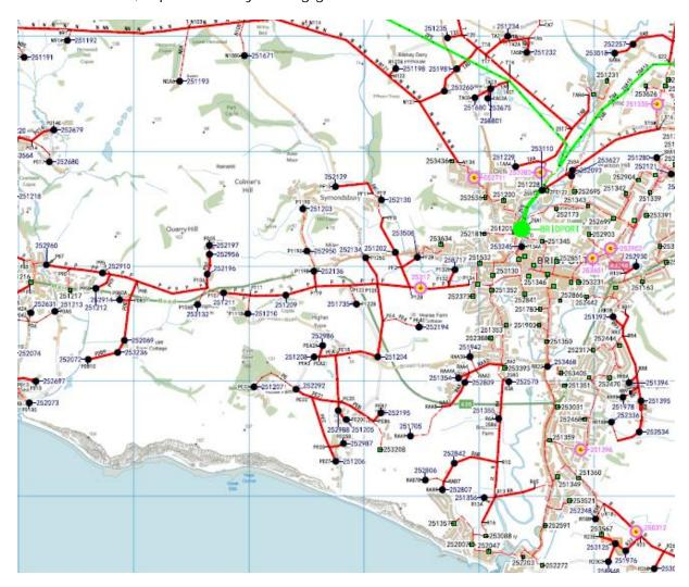
To ensure maximum flexibility in the network, some of the branching circuits connect with other circuits via some form of switch. Usually that switch is off (open) meaning no power can flow between the circuits. However in some circumstances such as faults on the network or maintenance, we may want to join circuits up to change the way power flows. This is done by turning switches on (closed) and connecting the circuits up.
