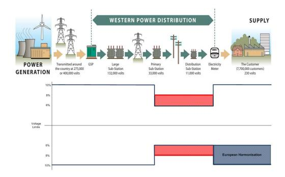
Figure 2 - Statutory voltage limits for operating GB's electricity networks
