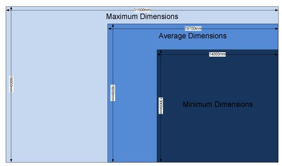
Figure 1 - 33kV FPL Dimensions
