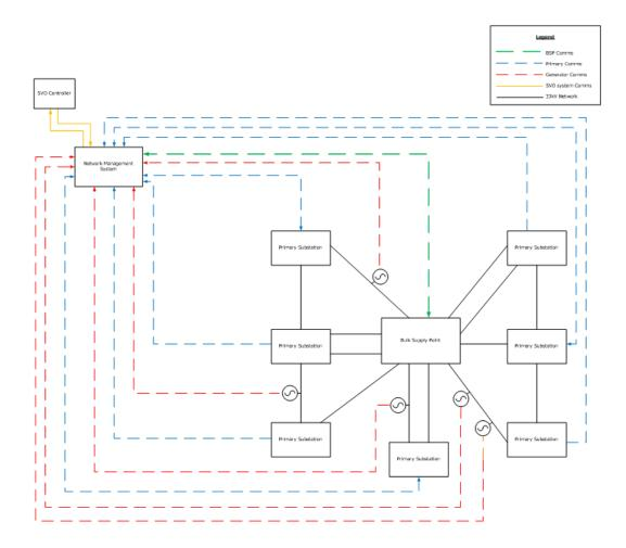
Figure 3 - System Voltage Optimisation Schematic
