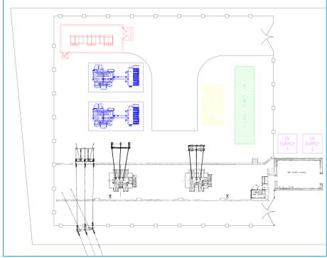
Figure 6-5: Proposed FPL and Switch House Layout for Exebridge
