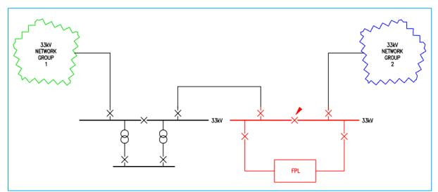
Figure 3-2: Option 1 - Proposed Network Arrangement
