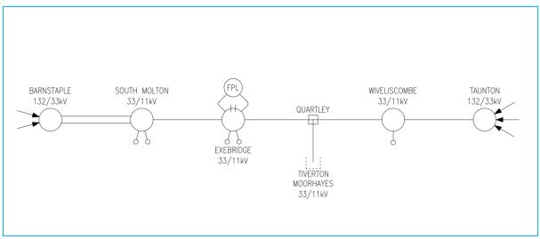
Figure 6-1: Overview of 33kV Network at Exebridge
