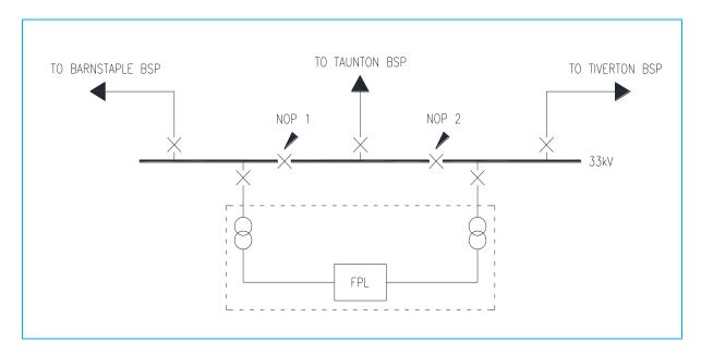
Figure 4-1: Proposed Quartley Single Line Diagram following the FPL Installation
