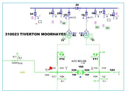
Figure 2-1: Existing Single Line Diagram
