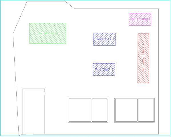
Figure 4-2: Proposed FPL and 33kV Switchhouse Layout at Tiverton Moorhayes
