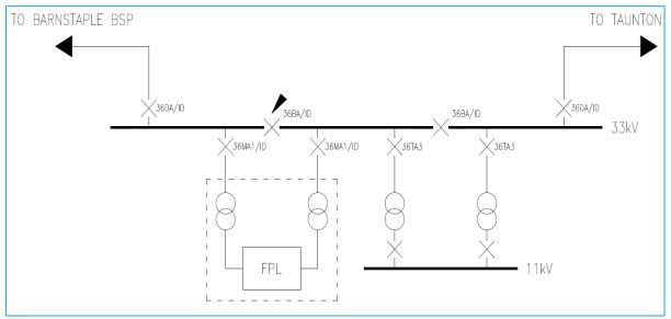
Figure 6-2: Exebridge 33/11kV Single Line Diagram following FPL Installation
