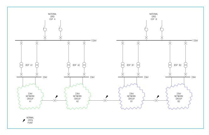
Figure 1-1: Typical Arrangement of a DNO Network
