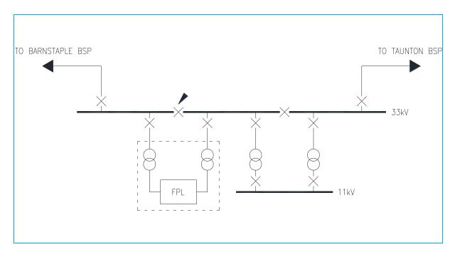
Figure 4-1: Proposed Exebridge 33/11kV Single Line Diagram Following the FPL Installation
