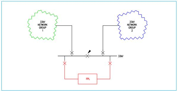
Figure 3-4: Option 2 – Across Existing Bus-Section Circuit Breaker
