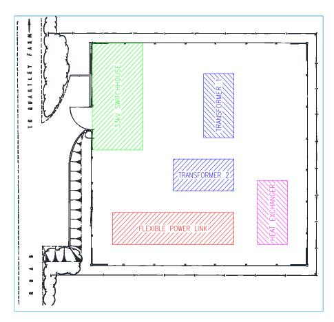
Figure 4-2: Proposed FPL and 33kV Switchhouse Layout at Quartley
