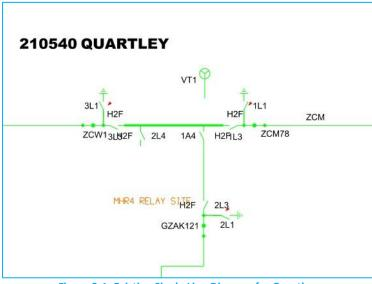
Figure 2-1: Existing Single Line Diagram for Quartley
