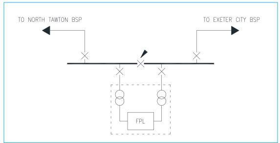
Figure 4-1: Proposed Winslakefoot Single Line Diagram following the FPL Installation
