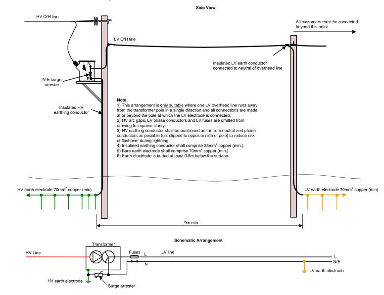
Figure 28Segregated HV and LV Earthing at Pole Mounted Substations<br/>- LV Earth Connected One Span from the Transformer Pole
