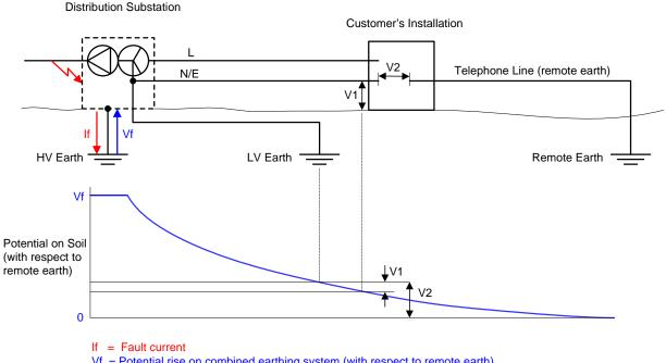
Vf = Potential rise on combined earthing system (with respect to remote earth)
