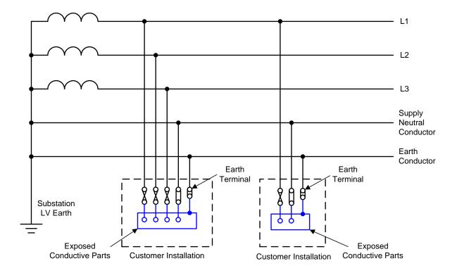
Figure 41 Separate Neutral and Earth (SNE)
