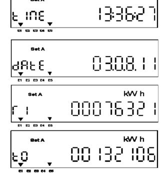
MD, Export, kVAh and kVArh registers are stored on Set B registers. They can be obtained by holding down the SELECT button for 3 seconds this switches the meter between Set A registers and Set B registers.
