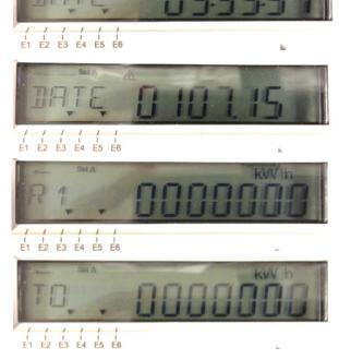
EW Export register is stored on Set B registers. They can be obtained by holding down the SELECT button for 3 seconds this switches the meter between Set A registers and Set B registers.
