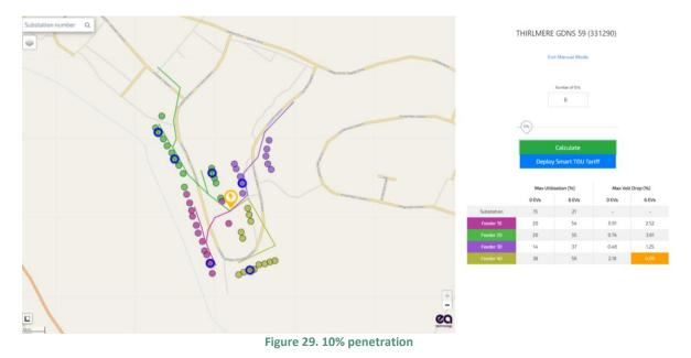
While the transformer is still operating within limits, Feeder 40 is now nearing a volt drop constraint as its approaching 5% on the main.
