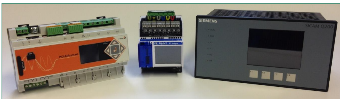
Figure 2-5 – The three PQ monitors being used for the project, from left to right: the a-eberle PQI-DA smart, the PSL PQube3, and the Siemens SICAM Q200
