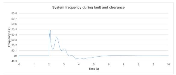
Figure 2-24 Frequency during fault and clearance - Min load
