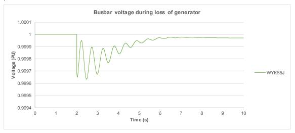
Figure 3.3 Voltage response after loss of a generator on EM1
