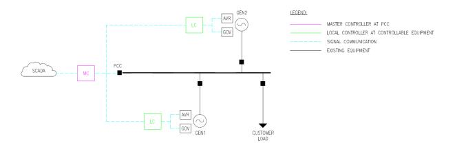
Figure 2.2 High-level island control system
