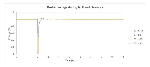
Figure 2-21 Busbar voltage during fault and clearance – Max load
