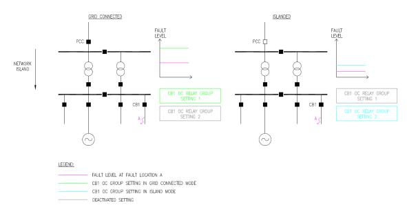
Figure 2.1 Overcurrent group settings in grid-connected and island modes
