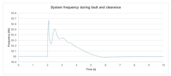
Figure 2-22 Frequency during fault and clearance – Max load
