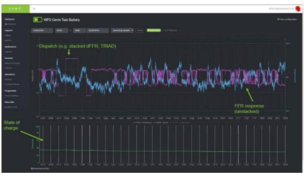
Figure 7: Illustration of FFR on the KiwiPower platform
