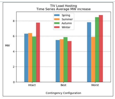
Figure 7-6 - Tiverton 33kV BSP time series average load hosting increase (MW)
