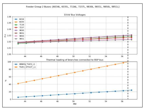
Figure 5-2 - Tiverton BSP 33 kV feeder group 2 with increasing generation
