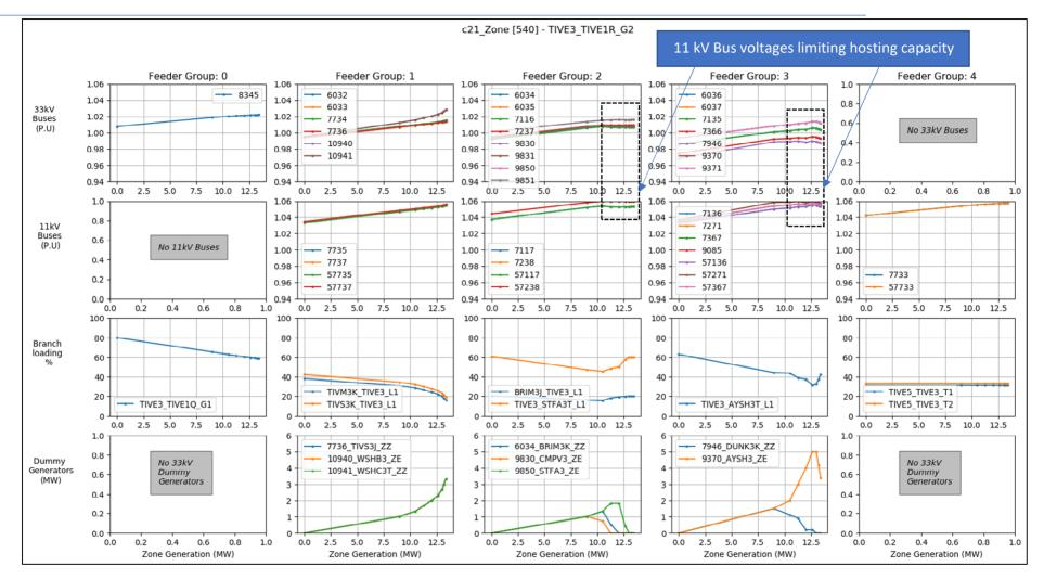
Figure 4-2 - Generation hosting algorithm for a contingency of Tiverton 132/33 kV transformer with fixed taps
