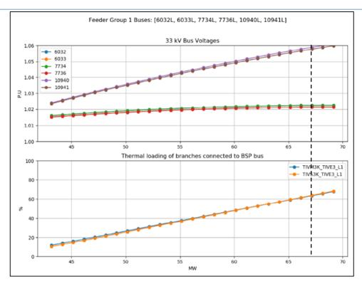
Figure 5-1 - Tiverton BSP 33 kV feeder group 1 with increasing generation
