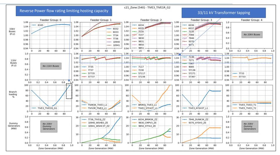
Figure 4-3 - Generation hosting algorithm for a contingency of Tiverton 132/33 kV transformer with tie transformers taps
