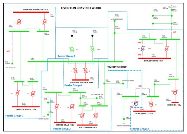
Figure 3-1 - Tiverton 33 kV BSP Feeder Groups
