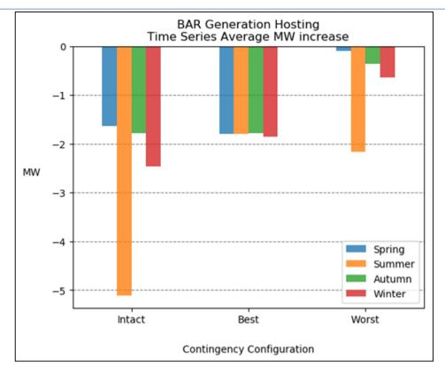
Figure 7-8 - Barnstaple 33kV BSP time series average generation hosting increase (MW)
