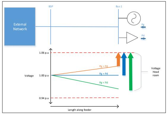
$\circ$  When the real power of the generator is greater than the load. (Pg > Pd)
