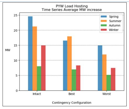
Figure 7-14 - Pyworthy and North Tawton 33kV BSP time series average load hosting increase (MW)
