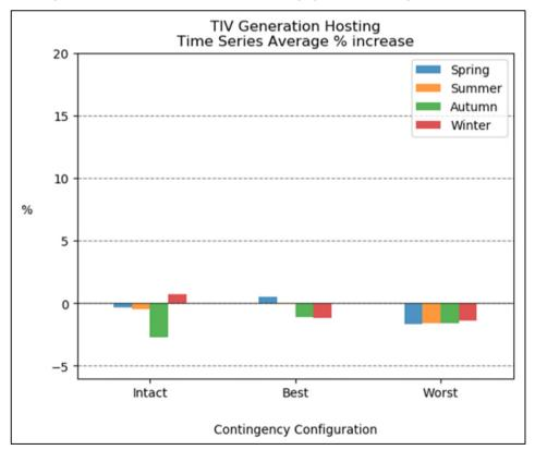
Figure 7-5 - Tiverton 33kV BSP time series average generation hosting increase (%)
