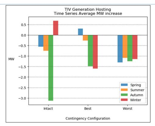
Figure 7-4 - Tiverton 33kV BSP time series average generation hosting increase (MW)
