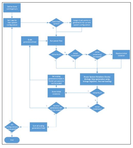
Figure 4-1 - Generation or Load Hosting per contingency algorithm process
