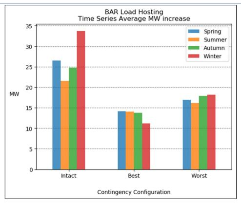
Figure 7-10 - Barnstaple 33kV BSP time series average load hosting increase (MW)
