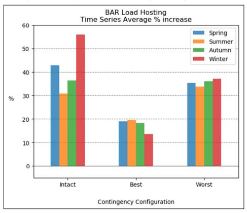
Figure 7-11 - Barnstaple 33kV BSP time series average load hosting increase (%)
