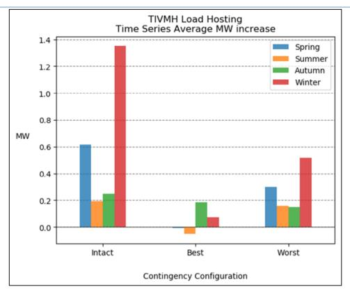
Figure 7-18 - Tiverton Moorhayes 11 kV Primary time series average load hosting increase (MW)
