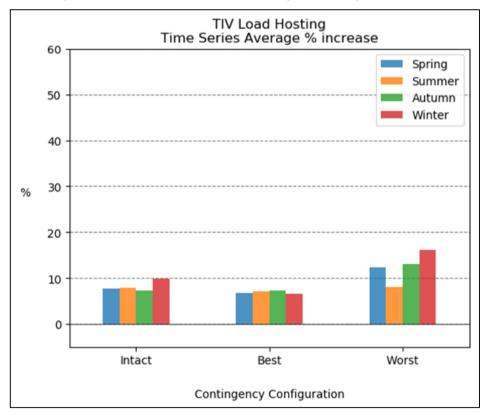
Figure 7-7 - Tiverton 33kV BSP time series average load hosting increase (%)
