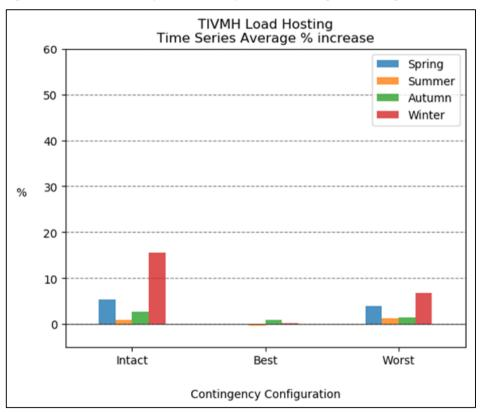
Figure 7-19 - Tiverton Moorhayes 11 kV Primary BSP time series average load hosting increase (%)
