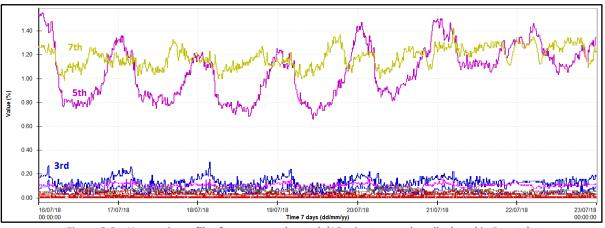
Figure 2-3 – Harmonic profiles for an example week (10 minute samples, displayed in Pronto).
