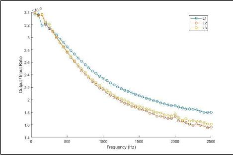
Figure 2-9 – Harmonic frequency response for the 3-phase 33 kV pole-mount outdoor VT.
