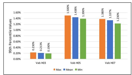
Figure 2-5 – Summary of effect on harmonic summary statistics by changing the start date and time of a standard weeklong monitoring window (Vab, based on 10 minute interval data).
