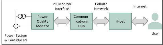
Figure 2-11 – Summary of overall architecture for PNPQA PQ monitoring and communication.
