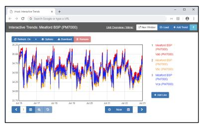
Figure 2-2 – Monitored voltage profiles for an example week viewed on iHost.
