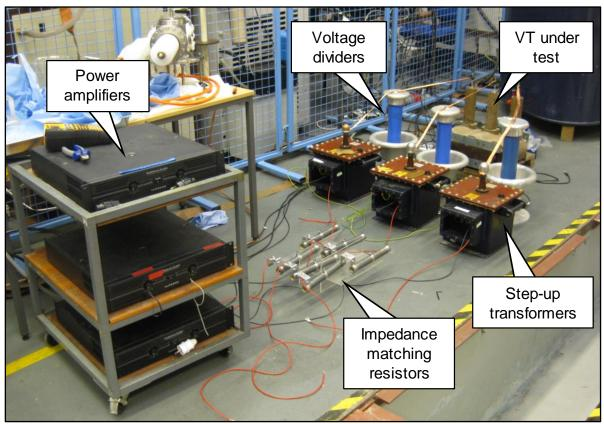
Figure 2-7 – VT testing circuit set up in The University of Manchester.
