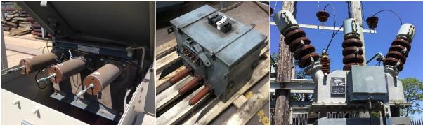
Figure 2-6 – VTs from within WPD used for testing. From left to right: 3-phase 11 kV VT from a metering unit; 3-phase 11 kV VT from a withdrawable switchgear panel; 3-phase 33 kV pole-mount outdoor VT.
