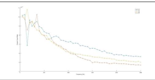
Figure 2-8 – Harmonic frequency response for the 3-phase 11 kV VT from a metering unit.
