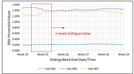
Figure 2-4 – Effect on voltage harmonic summary statistics (95<sup>th</sup> percentile values) by changing the start date and time of a standard week-long monitoring window (Vab, based on 10 minute interval data).
