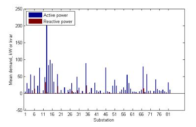
Mean distribution substation loads for substations supplied by the HV feeder. In this case emphasising the high number of connected transformers.
