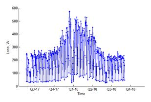
Figure 100 Long term mean daily (I<sup>2</sup>R) loss (Braddan I&C LV feeder)
