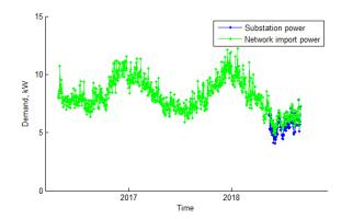
Figure 71 Long term mean daily feeder demand (Domestic Pilot LV feeder)
