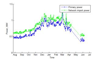
Figure 63 Long term mean daily feeder demand (Silver End HV feeder)
