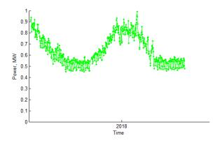
Figure 51 Long term mean daily feeder demand (Ackerman Tongwell Aldrich Drive Tee HV feeder)
