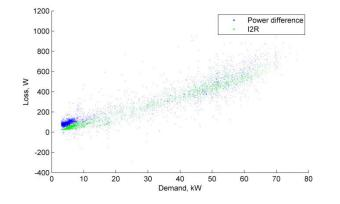
Figure 101 Aug 2018 Loss, kW vs demand, 10 min. av. (Braddan I&C LV feeder)
