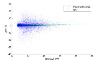
Figure 106 Aug 2018 Loss, % vs demand, 1 min. av. (Santon OH LV feeder)
