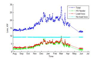
Figure 64 Long term mean daily (I<sup>2</sup>R) loss (Silver End HV feeder)
