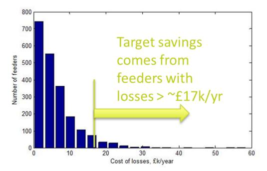
Figure 19 Cost of feeder losses histogram showing £17k/yr. threshold.
