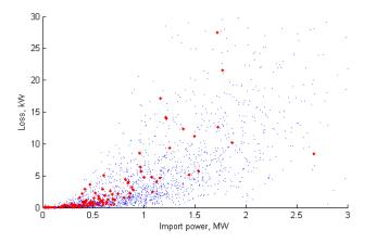
Figure 12 Line loss vs. network import power coloured for voltage (blue: 11 kV, red 6.6 kV).
