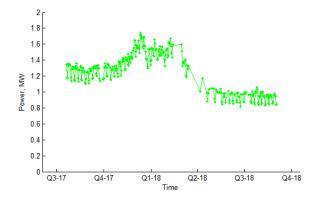
Figure 55 Long term mean daily feeder demand (The Avenue HV feeder)
