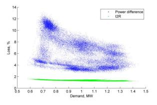
Figure 58 Aug 2018 Loss, % vs demand (The Avenue HV feeder)
