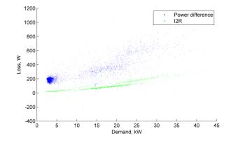
Figure 97 Aug 2018 Loss, kW vs demand, 10 min. av. (Ballasalla I&C LV feeder)
