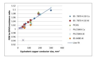
Figure 115 AC resistance scaling for underground cables.
