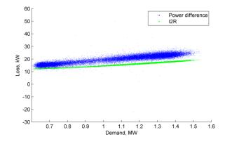
Figure 61 Aug 2018 Loss, kW vs demand (Riverside Park HV feeder)
