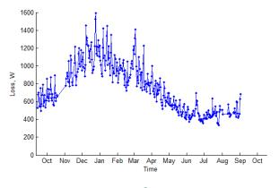
Figure 84 Long term mean daily (I<sup>2</sup>R) loss (Tromode Dom. LV feeder)
