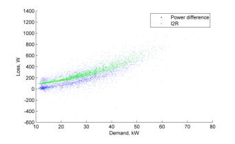
Figure 77 Aug 2018 Loss, kW vs demand, 10 min. av. (Laxey Dom. LV feeder)
