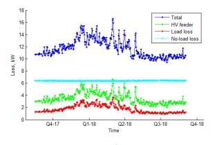
Figure 68 Long term mean daily (I<sup>2</sup>R) loss (Wolverton HV feeder)
