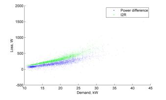
Figure 109 Aug 2018 Loss, kW vs demand, 10 min. av. (Abbeylands OH LV feeder)
