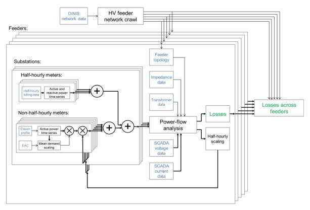
Figure 1 Outline of HV feeder loss estimation method.
