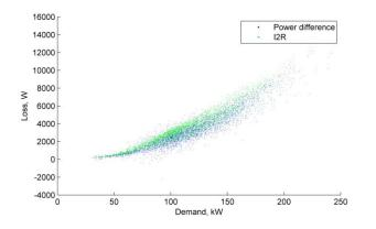
Figure 93 Aug 2018 Loss, kW vs demand, 10 min. av. (Peel B I&C LV feeder)
