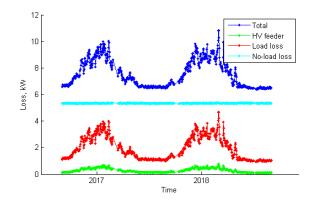
Figure 36 Long term mean daily (I<sup>2</sup>R) loss (Wavendon Gate Local HV feeder)
