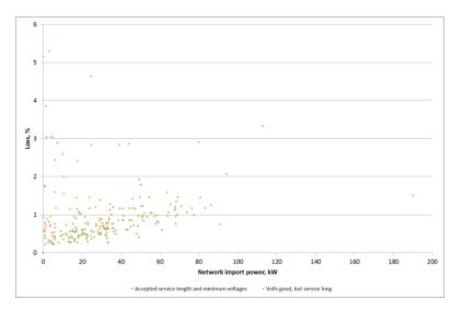
Figure 24 Loss percentage versus load scatter plot for "working" set of LV feeders.
