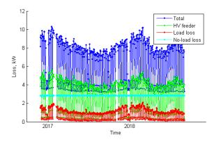
Figure 48 Long term mean daily (I<sup>2</sup>R) loss (Amway Tongwell HV feeder)
