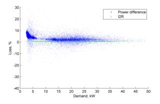
Figure 98 Aug 2018 Loss, % vs demand, 1 min. av. (Ballasalla I&C LV feeder)
