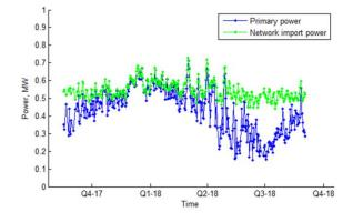
Figure 67 Long term mean daily feeder demand (Wolverton HV feeder)
