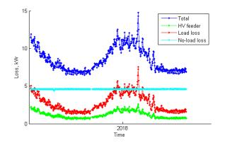
Figure 52 Long term mean daily (I<sup>2</sup>R) loss (Ackerman Tongwell Aldrich Drive Tee HV feeder)
