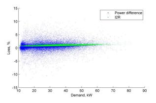
Figure 78 Aug 2018 Loss, % vs demand, 1 min. av. (Laxey Dom. LV feeder)
