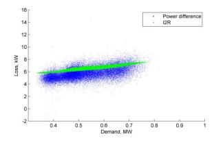
Figure 37 Aug 2018 Loss, kW vs demand (Wavendon Gate Local HV feeder)
