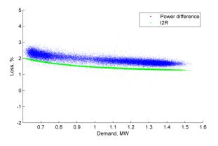
Figure 62 Aug 2018 Loss, % vs demand (Riverside Park HV feeder)
