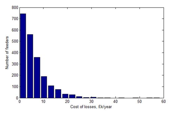
Figure 18 Cost of losses for feeders with accepted results, based on £48/MWh.
