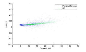
Figure 81 Aug 2018 Loss, kW vs demand, 10 min. av. (Ramsey Dom. LV feeder)
