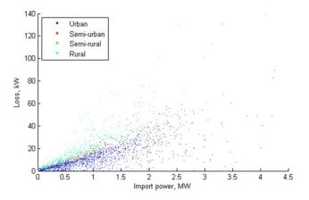
Figure 10 Loss vs. network import power coloured for feeder type.
