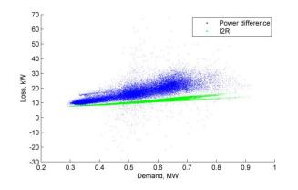
Figure 69 Aug 2018 Loss, kW vs demand (Wolverton HV feeder)
