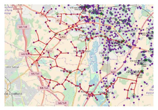
Figure 17 Feeder under review (shown with solid lines) and adjacent HV feeders (shown with dashed lines).
