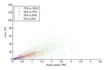
Figure 8 Loss vs. network import power coloured for proportion of losses due to transformer no-load losses.
