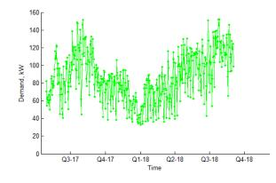
Figure 91 Long term mean daily feeder demand (Peel B I&C LV feeder)
