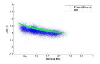
Figure 38 Aug 2018 Loss, % vs demand (Wavendon Gate Local HV feeder)
