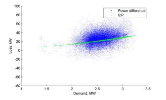
Figure 45 Aug 2018 Loss, kW vs demand (Crawley Road Tee Howard Way HV feeder)
