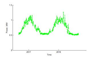
Figure 35 Long term mean daily feeder demand (Wavendon Gate Local HV feeder)
