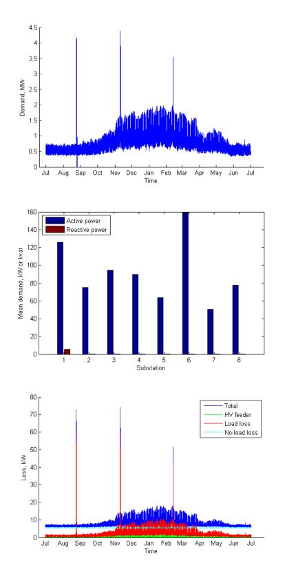
HV feeder demand. Spikes illustrate temporary changes in feeder configuration.
