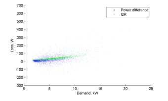
Figure 105 Aug 2018 Loss, kW vs demand, 10 min. av. (Santon OH LV feeder)
