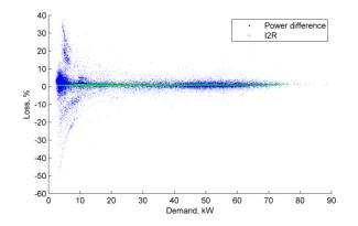
Figure 102 Aug 2018 Loss, % vs demand, 1 min. av. (Braddan I&C LV feeder)
