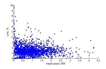
Figure 13 Revised losses scatter plot showing percentage loss versus feeder mean power.
