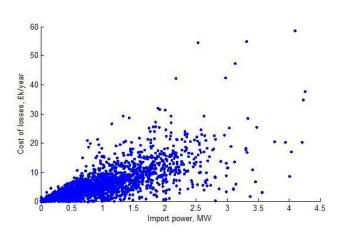
Figure 6 Cost of feeder losses vs. feeder load.
