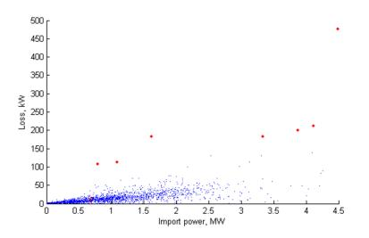
Figure 4 Scatter plot of mean loss power versus feeder mean power for HV feeders.
