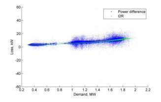
Figure 49 Aug 2018 Loss, kW vs demand (Amway Tongwell HV feeder)
