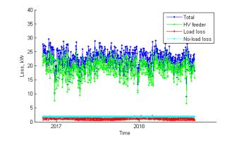
Figure 44 Long term mean daily (I<sup>2</sup>R) loss (Crawley Road Tee Howard Way HV feeder)
