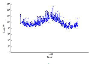
Figure 80 Long term mean daily (I<sup>2</sup>R) loss (Ramsey Dom. LV feeder)
