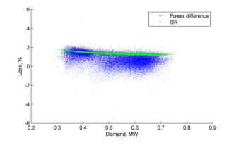
Figure 54 Aug 2018 Loss, % vs demand (Ackerman Tongwell Aldrich Drive Tee HV feeder)
