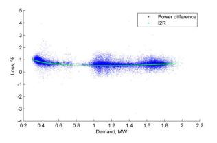
Figure 50 Aug 2018 Loss, % vs demand (Amway Tongwell HV feeder)
