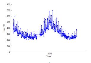
Figure 76 Long term mean daily (I<sup>2</sup>R) loss (Laxey Dom. LV feeder)
