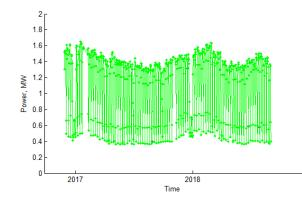
Figure 47 Long term mean daily feeder demand (Amway Tongwell HV feeder)
