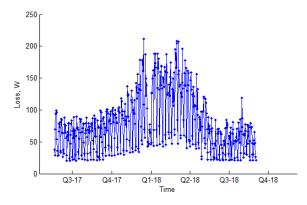
Figure 96 Long term mean daily (I<sup>2</sup>R) loss (Ballasalla I&C LV feeder)
