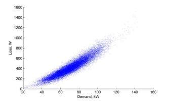
Figure 89 Aug 2018 2017 Loss, kW vs demand, 10 min. av. (Peel A I&C LV feeder)
