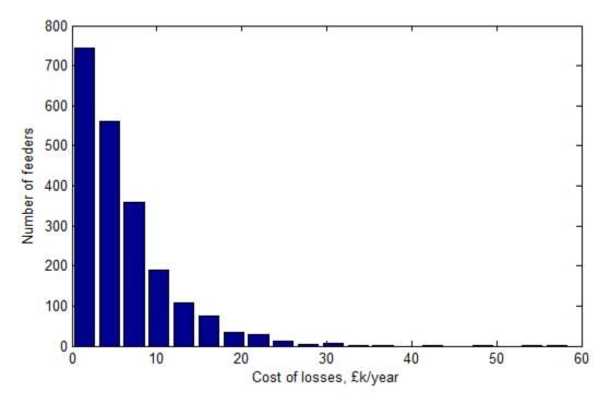
Figure 120 Cost of losses for feeders with accepted results, based on £48/MWh
