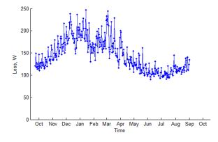
Figure 112 Long term mean daily (I<sup>2</sup>R) loss (Ramsey OH LV feeder)
