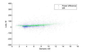
Figure 73 Aug 2018 Loss, kW vs demand, 10 min. av. (Dom. Pilot LV feeder)
