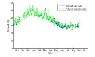
Figure 83 Long term mean daily feeder demand (Tromode Dom. LV feeder)
