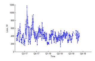
Figure 88 Long term mean daily (I<sup>2</sup>R) loss (Peel A I&C LV feeder)
