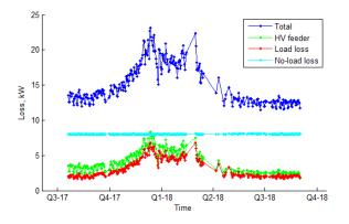
Figure 56 Long term mean daily (I<sup>2</sup>R) loss (The Avenue HV feeder)
