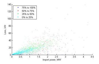
Figure 9 Loss vs. network import power coloured for proportion of losses due to HV cable load losses.
