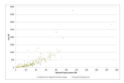
Figure 23 Loss power versus load scatter plot for "working" set of LV feeders.
