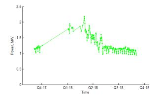
Figure 59 Long term mean daily feeder demand (Riverside Park HV feeder)
