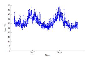
Figure 72 Long term mean daily (I<sup>2</sup>R) loss (Domestic Pilot LV feeder)
