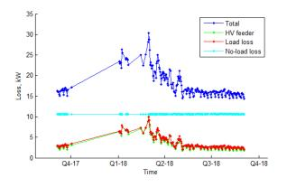
Figure 60 Long term mean daily (I<sup>2</sup>R) loss (Riverside Park HV feeder)
