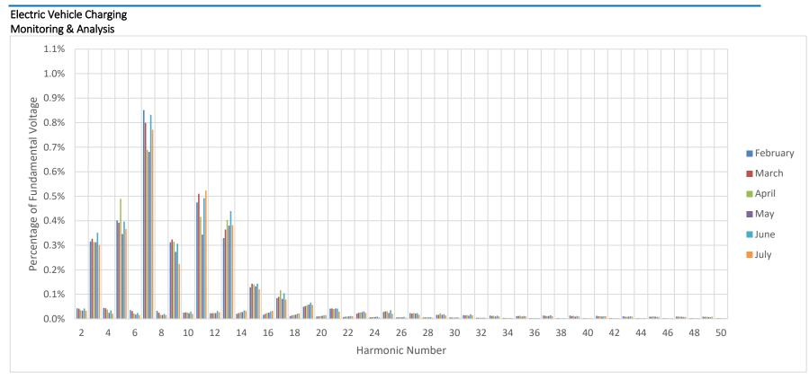
Figure 3-3: Background harmonic distortion on phase 3 during testing period
