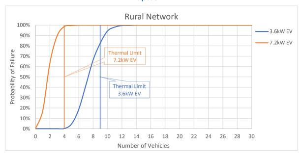
Figure C-8: Rural network with upper quartile EV profile, 0% background harmonic distortion and Zh as per equation 2-1
