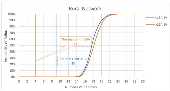
Figure C-11: Rural network with median EV profile, 0% background harmonic distortion and Z<sub>h</sub> as per equation 2-2
