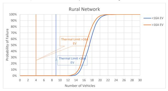
Figure 4-3: Rural network with typical median EV harmonic current, WPD background harmonic distortion and Z<sub>h</sub> calculated as per equation 2-2
