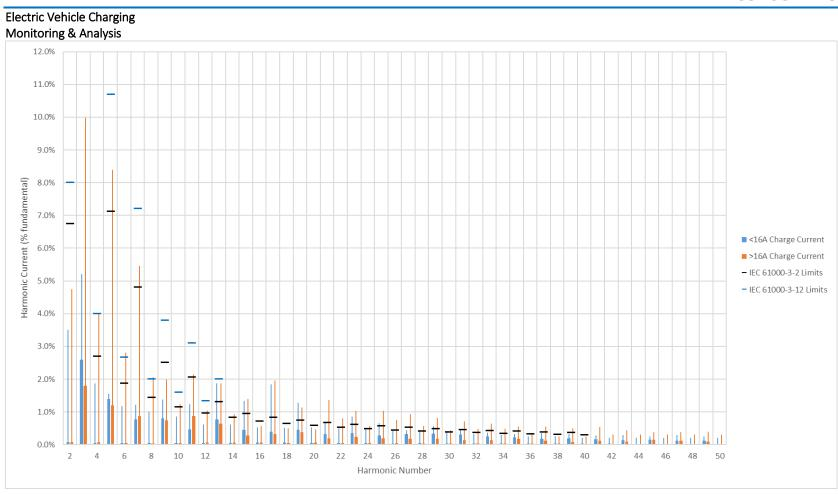
Figure 3-6: Median typical EV harmonic current assumed for <16 A and >16 A charge currents
