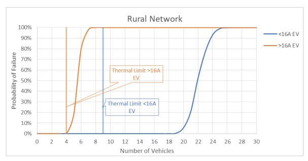
Figure 4-6: Rural network with a maximum source impedance of 0.21+j0.126 Ω with typical upper quartile EV harmonic current, WPD background harmonic distortion and Z<sub>h</sub> calculated as per equation 2-2
