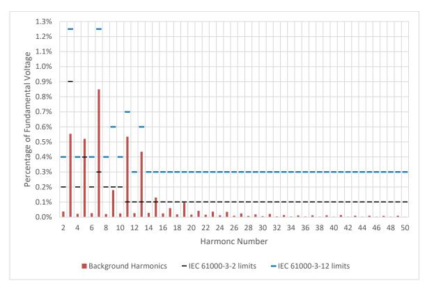
Figure 3-4: Average background voltage distortion compares against IEC 61000-3-2 and -12 limits
