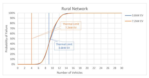
Figure C-5: Rural network with typical median EV harmonic current, WPD background harmonic distortion and Z<sub>h</sub> calculated as per equation 2-1
