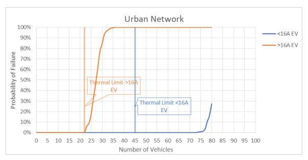
Figure 4-5: Urban network with a maximum source impedance of 0.127+j0.068  $\Omega$  with typical upper quartile EV harmonic current, WPD background harmonic distortion and Z<sub>h</sub> calculated as per equation 2-2
