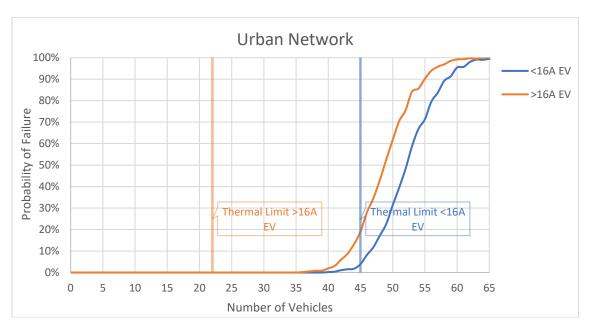
Figure 4-1: Urban network with median EV profile, WPD background harmonic distortion and Z<sub>h</sub> as per equation 2-2
