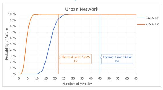
Figure C-4: Urban network with upper quartile EV profile, 0% background harmonic distortion and Z<sub>h</sub> as per equation 2-1
