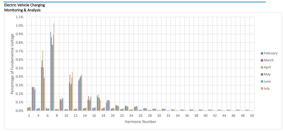
Figure 3-2: Background harmonic distortion on phase 2 during testing period
