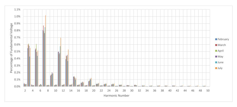
Figure 3-1: Background harmonic distortion on phase 1 during testing period
