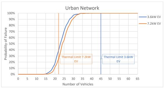
Figure C-3: Urban network with median EV profile, 0% background harmonic distortion and Z<sub>h</sub> as per equation 2-1
