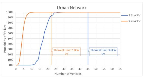
Figure C-2: Urban network with typical upper quartile EV harmonic current, WPD background harmonic distortion and Z<sub>h</sub> calculated as per equation 2-1
