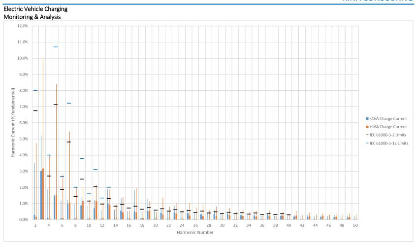
Figure 3-7: Upper quartile typical EV harmonic current for <16 A and >16 A charging currents
