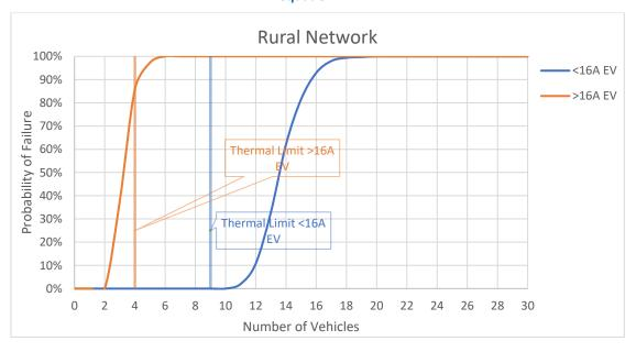
Figure C-12: Rural network with upper quartile EV profile, 0% background harmonic distortion and Z<sub>h</sub> as per equation 2-2
