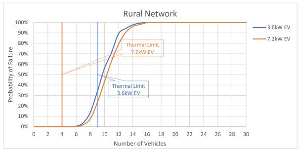
Figure C-7: Rural network with median EV profile, 0% background harmonic distortion and Z<sub>h</sub> as per equation 2-1
