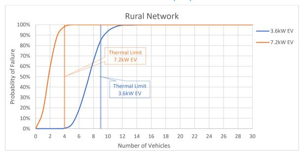
Figure C-6: Rural network with typical upper quartile EV harmonic current, WPD background harmonic distortion and Z<sub>h</sub> calculated as per equation 2-1
