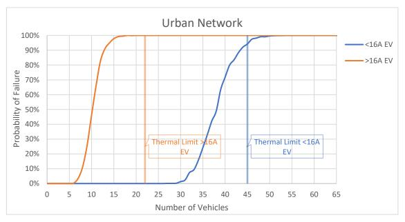
Figure 4-2: Urban network with upper quartile EV profile, WPD background harmonic distortion and Z<sub>h</sub> as per equation 2-2
