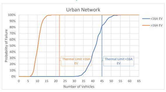
Figure C-10: Urban network with upper quartile EV profile, 0% background harmonic distortion and Z<sub>h</sub> as per equation 2-2
