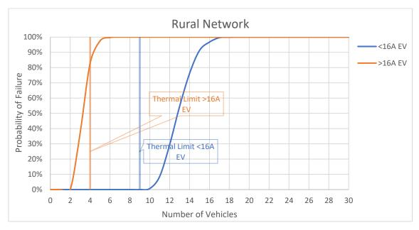
Figure 4-4: Rural network with typical upper quartile EV harmonic current, WPD background harmonic distortion and Z<sub>h</sub> calculated as per equation 2-2
