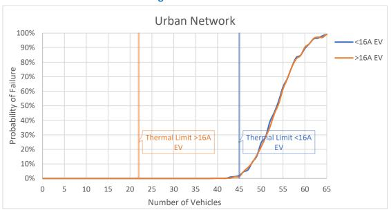
Figure C-9: Urban network with median EV profile, 0% background harmonic distortion and Z<sub>h</sub> as per equation 2-2
