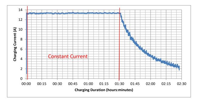
Figure 2-2: Typical 3.2 kW charging profile with extracted constant current section marked
