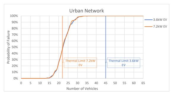
Figure C-1: Urban network with typical median EV harmonic current, WPD background harmonic distortion and Z<sub>h</sub> calculated as per equation 2-1
