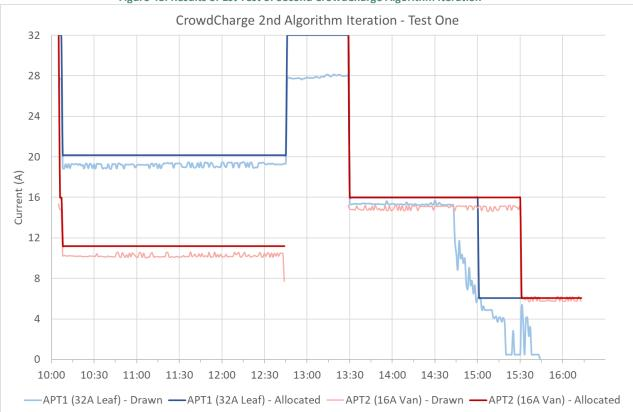
Figure 48: Results of 1st Test of Second CrowdCharge Algorithm Iteration
