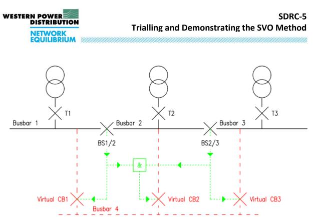
Figure 2-23: SuperTAPP SG Virtual Busbar Concept
