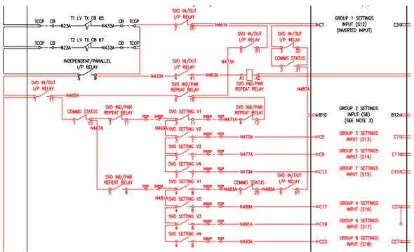
Figure 2-17: MircoTAPP Relay Interface Logic
