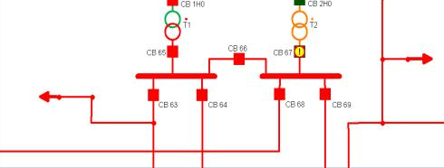
Figure 4-1 Waterlake CB 67 in DBI state
