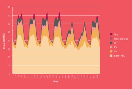
Figure 8. Electricity demand and equivalent heat pump gas demand.
