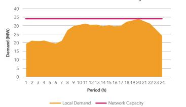
Figure 11. Local electricity demand at primary substation level and secured network capacity in a typical winter day.
