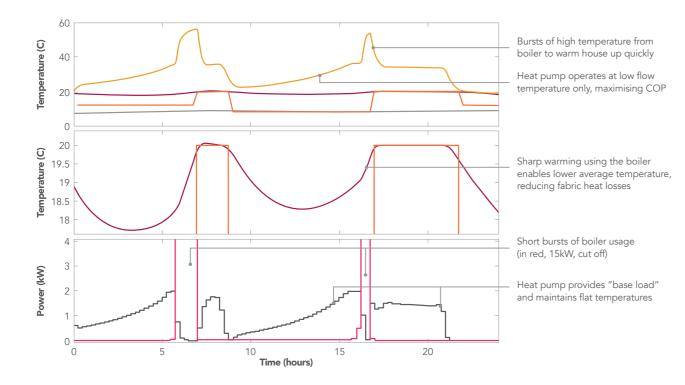
Figure 13. Graphs illustrating cost-optimised control of a hybrid system with a gas:electricity price ratio of 1:3, showing day-ahead predictions of heating water temperature (top), room temperature (middle), and power consumption (bottom, with electricity in black and gas in red).
