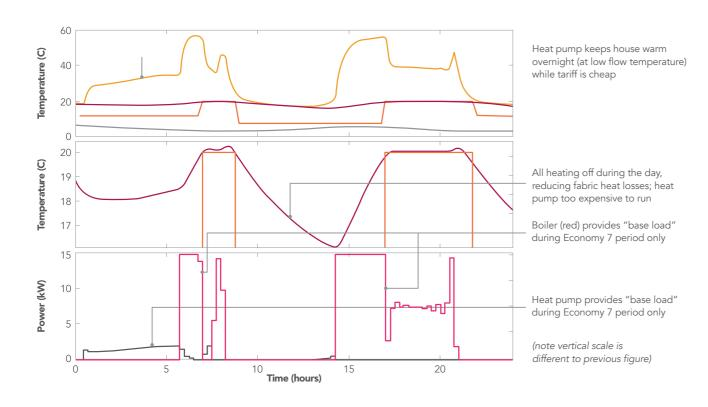
Figure 14. Graphs illustrating cost-optimised control of a hybrid system on an Economy 7 electricity and current (Oct 2016) prices, showing day-ahead predictions of heating water temperature (top), room temperature (middle), and power consumption (bottom, with electricity in black and gas in red).
