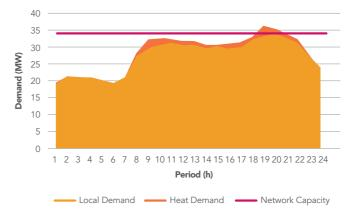
Figure 12. Local and electrified heat demand at the distribution network (a) without and (b) with network support service.
