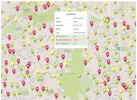
Figure 1 – Example transformer location map from the NAT (mocked up data showing transformer grading by an "EV Impact" rating for illustration purposes)
