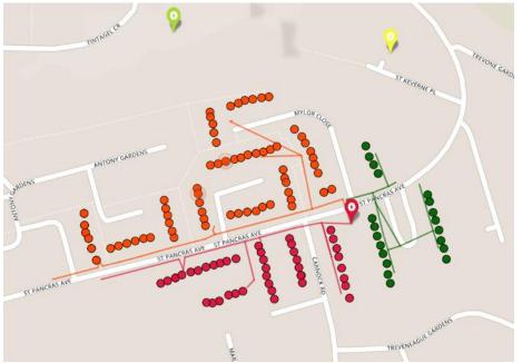
Figure 2 – Example feeder map developed by the heuristics, colours indicate association from the NAT
