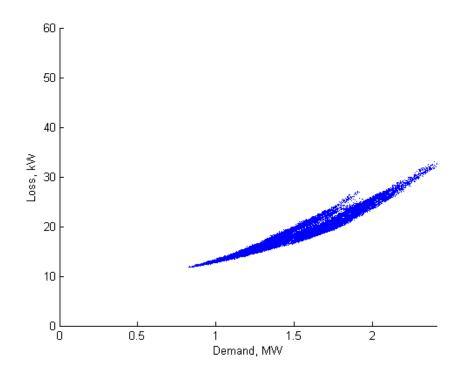
Figure 11 Pilot HV feeder losses for each 1 minute sample calculated with I<sup>2</sup>R method
