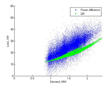
Figure 13 Pilot HV feeder losses for each 1 minute sample calculated with the power difference method and with the I<sup>2</sup>R method
