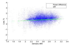
Figure 33 March 2017 Loss, % vs demand (Crawley Road Tee Howard Way HV feeder)
