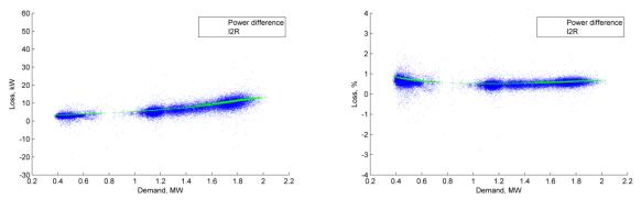
Figure 7 March 2017 Loss, kW vs demand (Amway F Tongwell HV feeder)
