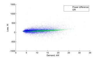
Figure 44 March 2017 Loss, kW vs demand (Domestic Pilot LV feeder)
