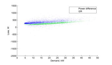
Figure 52 March 2017 Loss, kW vs demand (Ramsey Domestic LV feeder)
