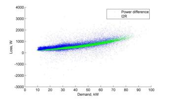
Figure 48 March 2017 Loss, kW vs demand (Laxey Domestic LV feeder)
