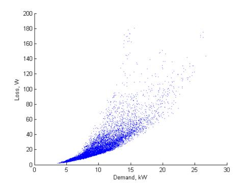
Figure 12 Pilot LV feeder losses for each 1 minute sample calculated with I2R method
