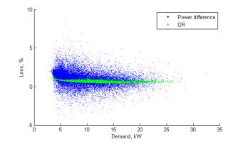
Figure 45 March 2017 Loss, % vs demand (Domestic Pilot LV feeder)
