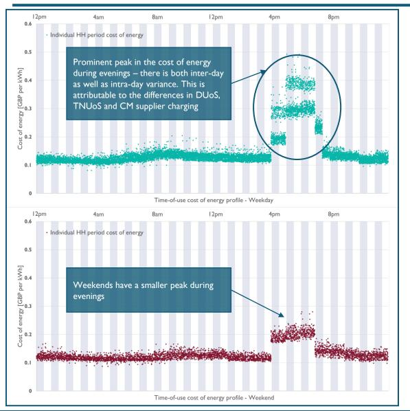
The cost of energy (ie., the wholesale energy price plus network charges plus nonenergy charges) is used as the price signal for the customer energy cost. A halfhourly timeseries for a full year has been used in the modelling, and is made up of the following components:
