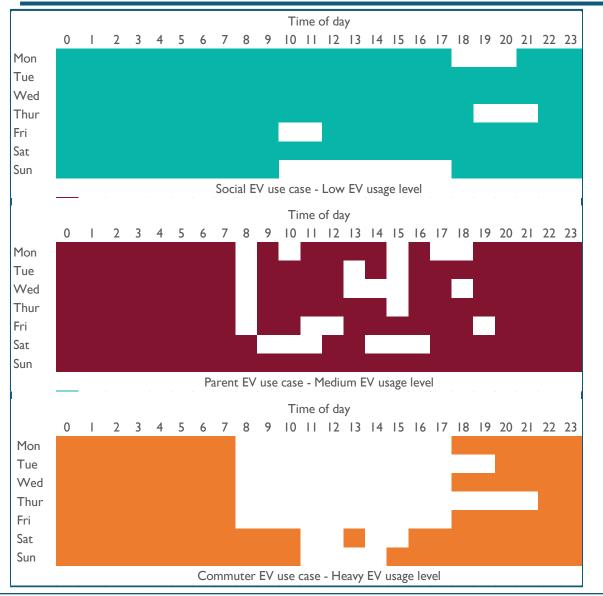
The images show the EV transport pattern used in the modelling for each customer type as provided by Delta-ee. Delta-ee has noted that the transport patterns are informed by National Transport Statistics (2018 update) as well as BEIS CP data. Similar to the customer load data, the transport pattern data are provided as a representative weekday and weekend profile, which is then applied across the full year for modelling.
