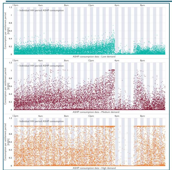
The graphs show the ASHP electrical load data used in the modelling for each customer type. These data are an output from the hybrid heating system optimisation completed by PassivSystems based on 2018 heating profile data for a selection of homes from the Freedom Project.
