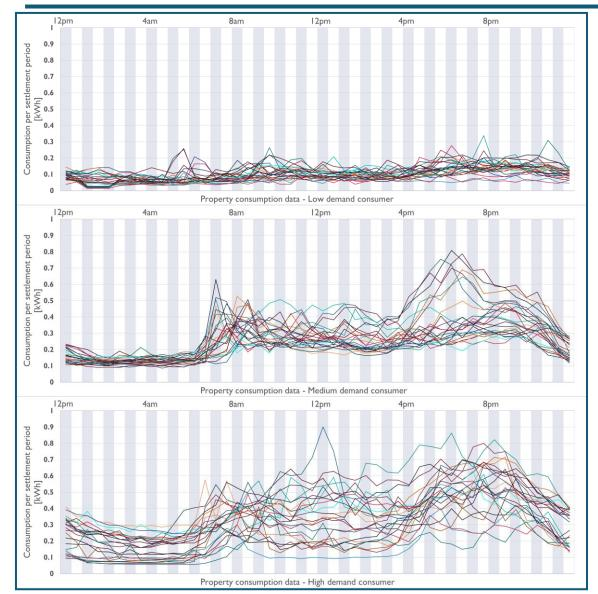
The graphs show the consumer load data used in the modelling for each customer type as provided by Delta-ee. The data does not included any electric heating loads.
