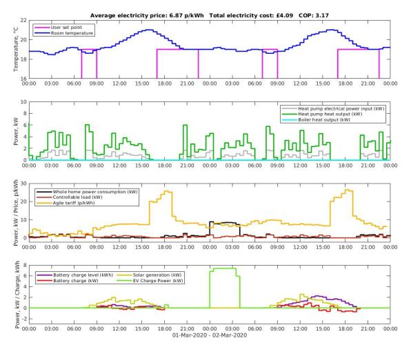
Figure 8.1 - Full simulation run under Phase 1 control with smart EV charging (Digital twin of Home 2, 01/03/2020 - 02/03/2020)
