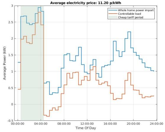
Figure 3.7 - Average load profiles for phase 2 operation on Octopus Go tariff (All homes, 18/02/2020 - 27/02/2020, note that three days worth of data were excluded from this range due to interventions which significantly affected the demand profile). Controllable load is the combination of heat pump and battery in this case. Whole home power import = import from (/export to) the grid.
