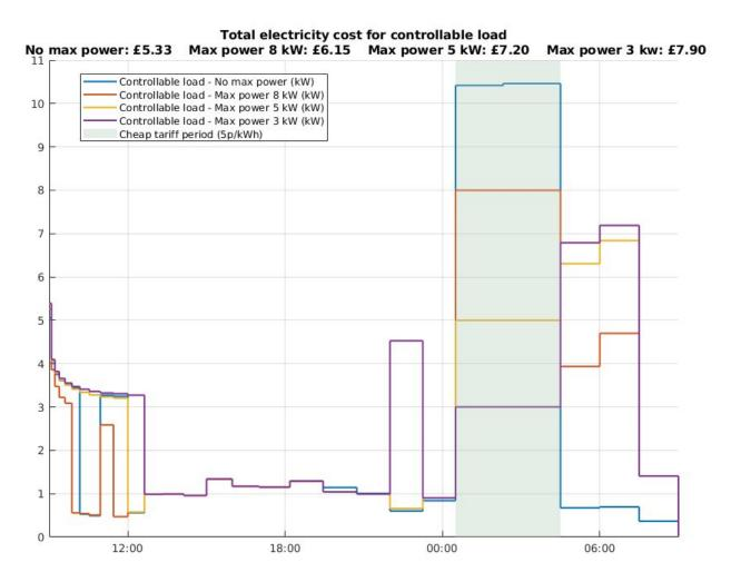
Figure 4.5 - Simulated controllable load on the Octopus Go tariff with a range of maximum power limits between 00:30 - 04:30 (Digital twin of Home 5, 03/01/2020 - 04/01/2020). Day tariff rate is 13.8p/kWh with a cheap overnight tariff rate of 5p/kWh as indicated on the figure.
