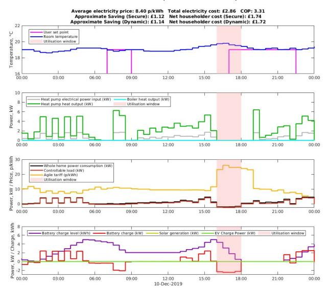
Figure 9.3 - Full simulation run, 16:00 - 18:00 request utilised on the Octopus Agile tariff (Digital twin of Home 2, 10/12/2019)
