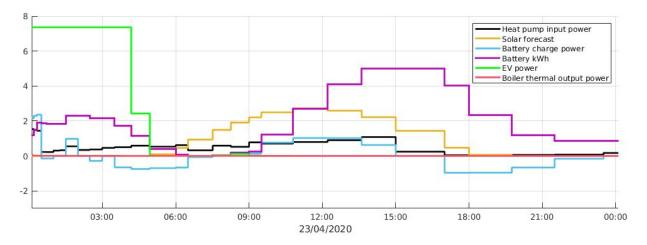
Figure 4.2 - Optimisation output under Phase 2 control (Digital twin of Home 5, 23/04/2020)
