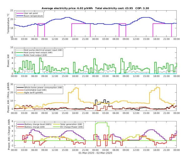
Figure 8.2 - Full simulation run under Phase 2 control with smart EV charging (Digital twin of Home 2, 01/03/2020 - 02/03/2020)
