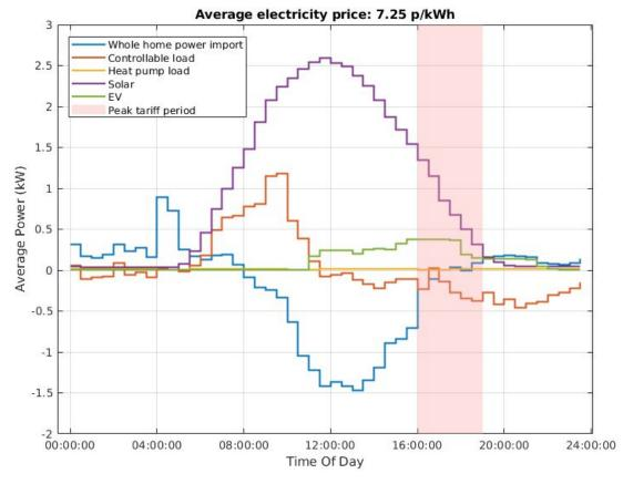
Figure 3.16 - Average load profiles for summertime operation on Octopus Agile tariff (All homes, 25/05/2020 - 01/06/2020). Controllable load refers to heat pump plus domestic battery plus EV charge. Whole home power import = import from (/export to) the grid.
