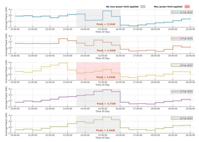
Figure 3.21 - Average controllable load (heat pump + battery load) over all MADE homes on Octopus Agile tariff (All homes, 12/02/2020 - 16/02/2020)
