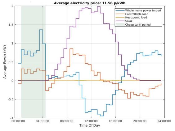
Figure 3.18 - Average load profiles for summertime operation on Octopus Go tariff (All homes, 17/07/2020 - 23/07/2020). Controllable load refers to heat pump plus domestic battery plus EV charge. Whole home power import = import from (/export to) the grid.
