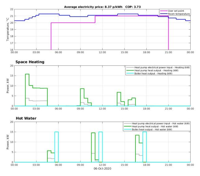
Figure 10.4 - Hot water intervention (Home 03, 06/10/2020). Note that the boiler heat output is estimated as this home does not have a boiler heat meter.
