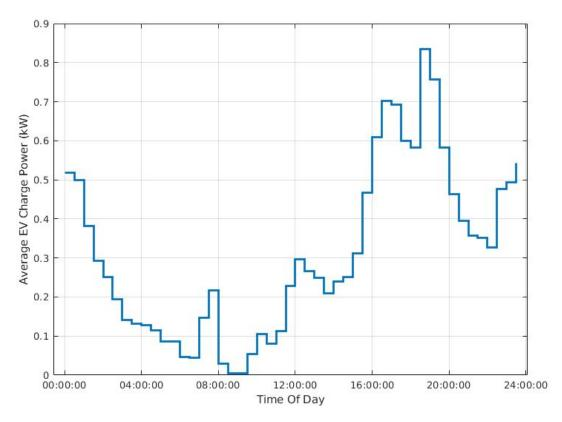
Figure 3.5 - Average EV charge power across the day for the MADE homes (Homes 2,3,4 & 5, 01/12/2019 - 15/01/2020. Note that Home 1 was not included in this analysis since the charge point was installed at a later date.)
