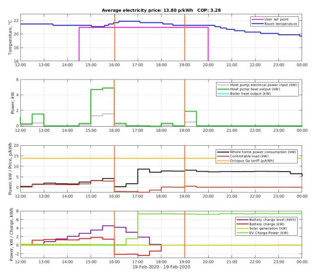
Figure 3.23 - Secure Flexible Power intervention (Home 2, 19/02/2020). Controllable load is the combination of heat pump and battery in this case.
