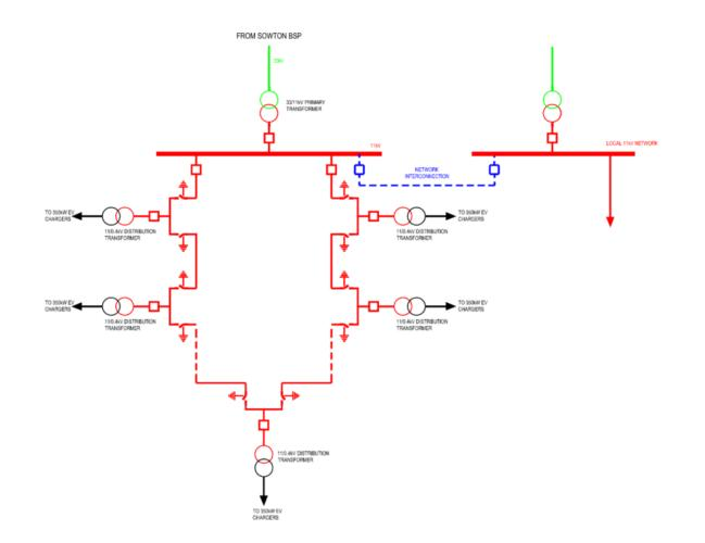
Figure 5-2 Example of network connection by single primary transformer and interconnection to local 11kV network for charging station
