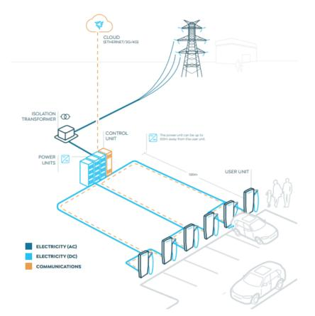
Figure 2-16 Example of system components for installation of Veefil PK 350kW chargers.
