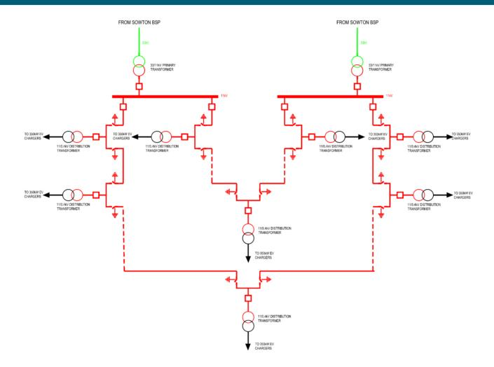
Figure 5-1 Example of network connection by two primary transformers for charging station
