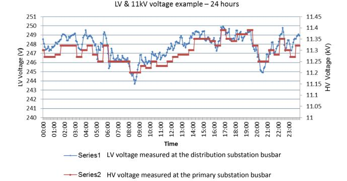
Figure 14 - LV and 11kV feeder voltage profile
