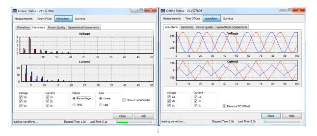
Figure -16 Effect of harmonics on the LV current and voltage wave forms
