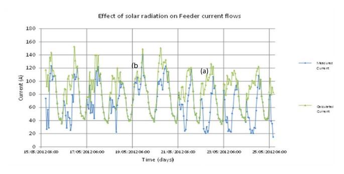
Figure - 12 Impact of solar PV on network current
