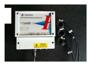
Figure 7 - Rogowski coil and transconductance amplifier Current transducer
