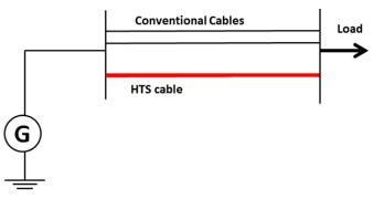
Figure 3.4: Conventional cables and superconducting cables working in parallel
