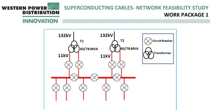
Figure 2.1 - Example 132/11kV substation
