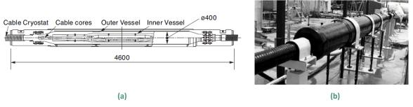
Figure 4.14: (a) Schematic view of "3-in-one" HTS joint. (b) Appearance of "3-in-one" HTS joint. [24]
