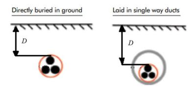
Figure 5.6: Schematic of depth of cover (D)
