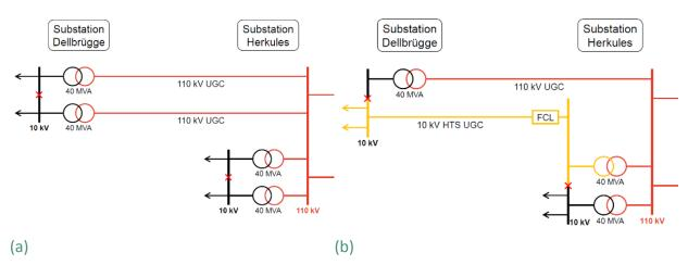
Figure 3.5: AmpaCity grid configuration (a) installation of conventional cable solution, (b) alternative installation of superconducting cable solution [16]
