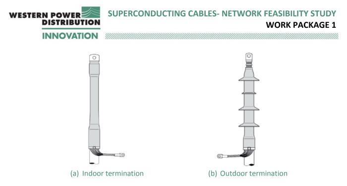
Figure 5.2: Schematic of indoor and outdoor terminations
