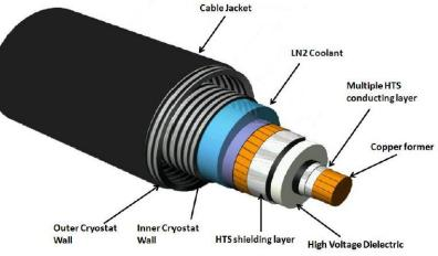
Figure 4.1: Single-phase superconducting cable. [4]
