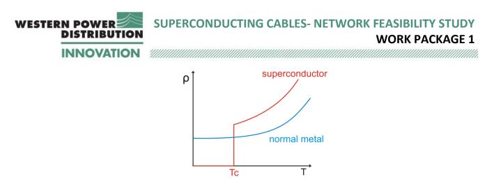
Figure 3.1: Critical temperature (Tc) of superconductor compared to normal metal
