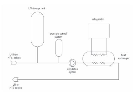
Figure 4.8: Structure of completed cryogenic cooling system.
