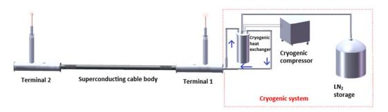
Figure 4.16: Schematic of superconducting cable cryogenic cooling system [32]
