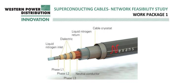
Figure 4.4: Configuration of the triaxial CD superconducting cable [4]
