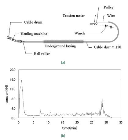
Figure 4.12: (a) Schematic of the HTS cable installation (b) Pulling tension of the cable into the duct measured by a tension meter at the outlet of the duct [22]
