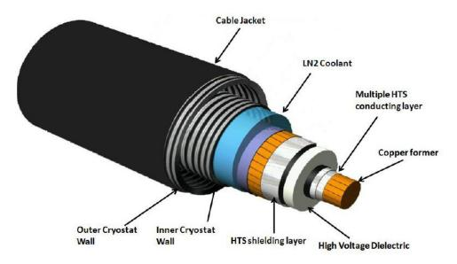
Figure 4.2 : Single-phase superconducting cable
