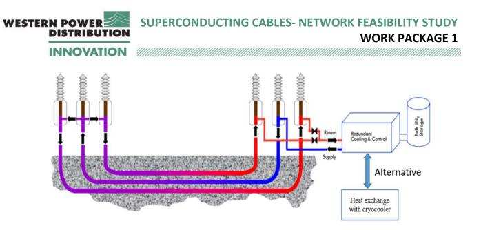
Figure 4.7: The self-circulating cooling system for superconducting cable. [7]
