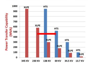
Figure 3.2: The power transmission capacity and voltage level of XLPE cable and superconducting cable. [10]
