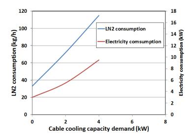
Figure 4.19: Liquid nitrogen (LN2) and electricity consumption of a completed 1 km superconducting cable system [47]
