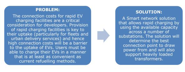
The Project will use an equalisation network to provide an alternative, cost-effective solution for rapid EV charging demands, more flexibly than a traditional AC reinforcement solution. The solution seeks to explore the comparative benefits of a DC network, where power flows can be actively managed, and fault level contained, over a traditional AC network reinforcement.
