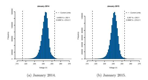
Figure 3.15: The frequencies of voltage values measured at all feeder ends.
