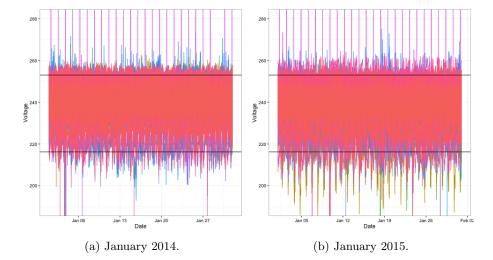
Figure 3.14: Voltage data measured at all feeder end monitors. Measurements are for each ten-minute periods in January 2014 and 2015. The black horizontal lines indicate the statutory limits of 230V + 10%, -6%.
