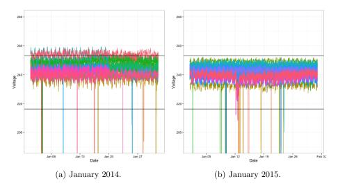
Figure 3.7: Ten-minute voltage data plotted for each substation where at least one ten-minute period is below the statutory limit, for January 2014 and 2015.
