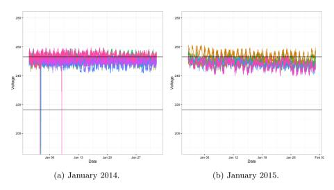
Figure 3.6: Ten-minute voltage data plotted for each substation where at least one ten-minute period exceeds the statutory limit, for January 2014 and 2015.
