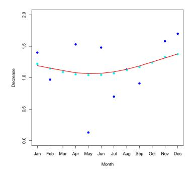
Figure 2.3: Estimates of the percentage decrease in average demand, by month. Comparisons are between 2014 and 2015. The dark blue dots indicate the estimates from a paired comparison by substation and the light blue dots a set of 'smoothed' estimates based on a lowess smoother (red line).
