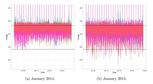
Figure 3.19: Ten-minute voltage data plotted for each monitor at feeder end where at least one ten-minute period exceeds the statutory limit, for January 2014 and 2015.
