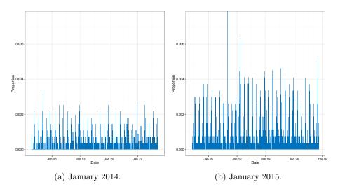
Figure 3.22: Proportion of monitors at feeder ends below the statutory limit in each ten-minute period in January 2014 and 2015.
