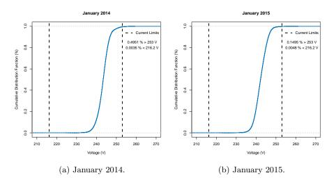
Figure 3.3: The cumulative distribution function for voltages measured at all substations.
