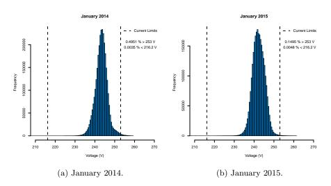
Figure 3.2: The frequencies of voltage values measured at all substations.
