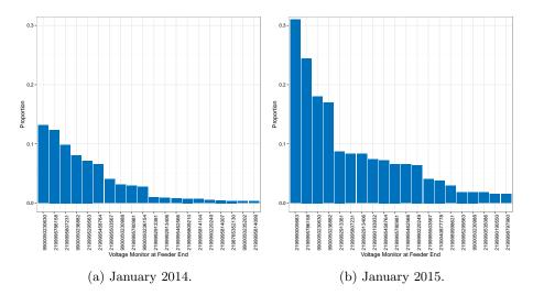
Figure 3.26: Proportion of ten-minute periods that a monitor at feeder end is below the statutory limit, for the twenty feeder end monitors with the most under-excursions, in January 2014 and 2015.
