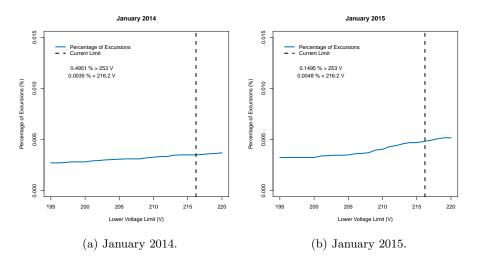
Figure 3.4: Excursions at the lower statutory limits for all substations in January 2014 and 2015. The current limit is marked by the black dashed line.
