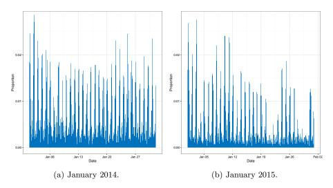
Figure 3.21: Proportion of monitors at feeder ends exceeding the statutory limit in each ten-minute period in January 2014 and 2015.
