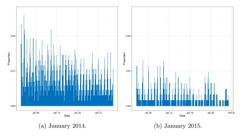
Figure 3.8: Proportion of substations exceeding the statutory limit in each tenminute period in January 2014 and 2015.
