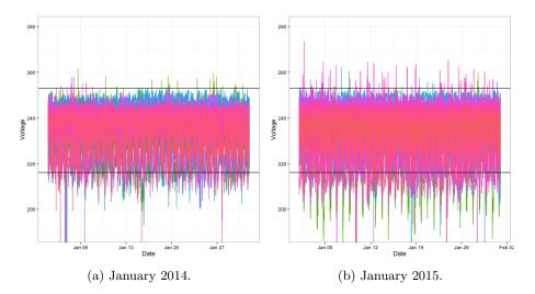
Figure 3.20: Ten-minute voltage data plotted for each monitor at feeder end where at least one ten-minute period is below the statutory limit, for January 2014 and 2015.
