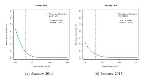
Figure 3.18: Excursions at the upper statutory limits for all feeder ends in January 2014 and 2015. The current limit is marked by the black dashed line.
