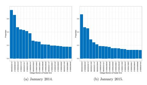
Figure 3.25: Proportion of ten-minute periods that a monitor at feeder end exceeds the statutory limit, for the twenty feeder end monitors with the most over-excursions, in January 2014 and 2015.
