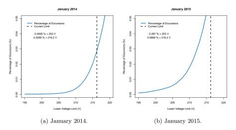
Figure 3.17: Excursions at the lower statutory limits for all feeder ends in January 2014 and 2015. The current limit is marked by the black dashed line.
