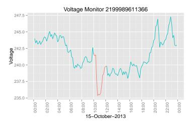
Figure 4.2: Demand profile for substation 511222 on October 15th, 2013, the day of the Operation Juniper trial during which voltages were dropped between 10:00am and 12:00pm.
