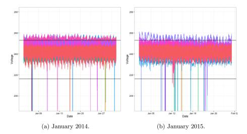
Figure 3.1: Voltage data measured at all substations. Measurements are for each ten-minute periods in January 2014 and 2015. The black horizontal lines indicate the statutory limits of 230V + 10%, -6%.
