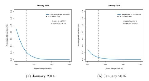
Figure 3.5: Excursions at the upper statutory limits for all substations in January 2014 and 2015. The current limit is marked by the black dashed line.
