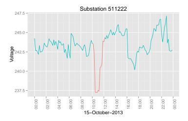
Figure 4.1: Voltage profile for substation 511222 on October 15th, 2013, the day of the Operation Juniper trial during which voltages were dropped between 10:00am and 12:00pm.
