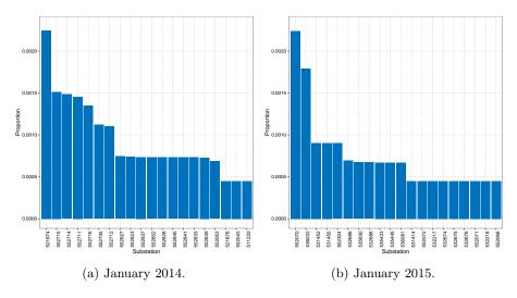
Figure 3.13: Proportion of ten-minute periods that a substation is below the statutory limit, for the twenty substations with the most under-excursions, in January 2014 and 2015.
