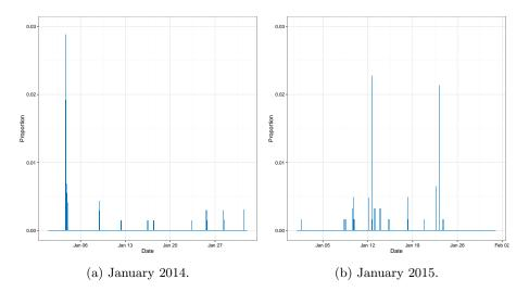
Figure 3.9: Proportion of substations below the statutory limit in each tenminute period in January 2014 and 2015.
