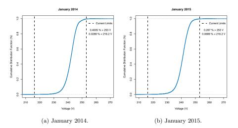
Figure 3.16: The cumulative distribution function for voltages measured at all feeder ends.
