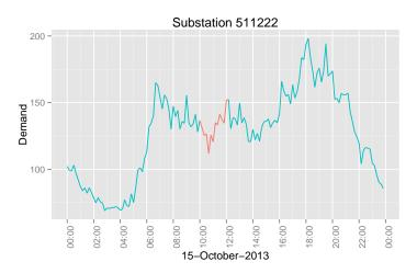
Figure 4.3: Demand profile for Substation 511222 on October 15th, 2013, the day of the Operation Juniper trial during which voltages were dropped between 10:00am and 12:00pm.
