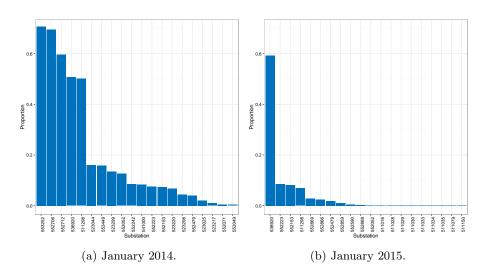
Figure 3.12: Proportion of ten-minute periods a substation exceeds the statutory limit, for the twenty substations with the most over-excursions, in January 2014 and 2015.
