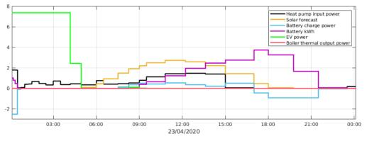
Figure 8: Optimisation output under Phase 1 control (Digital twin of Home 5, 23/04/2020)
