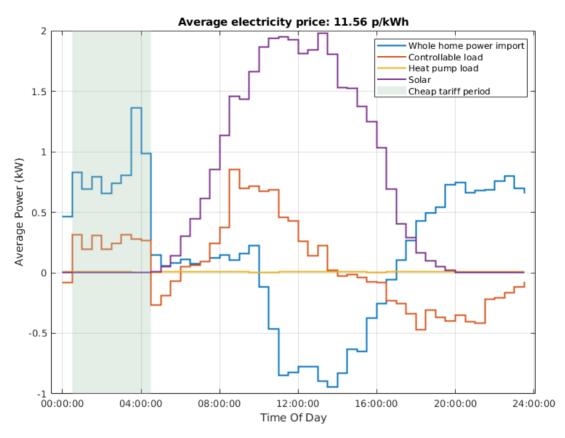
Figure 7: Average load profiles for summertime operation on Octopus Go tariff (All homes, 17/07/2020 - 23/07/2020). Controllable load refers to heat pump plus domestic battery plus EV charge. Whole home power import = import from (/export to) the grid.
