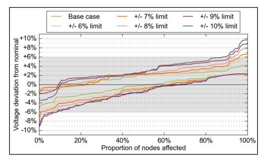
Figure 5: Cumulative frequency plots of steady state voltages for the high and low voltage cases when widened voltage limits are applied at 33kV (results from upstream model)
