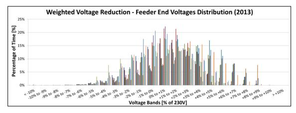
Figure 9: Distribution of reduced feeder end voltages
