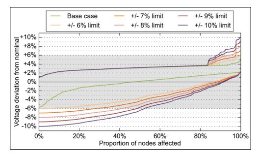
Figure 7: Cumulative frequency plots of steady state voltages for the high and low voltage cases when widened voltage limits are applied at 11kV (results from downstream model)
