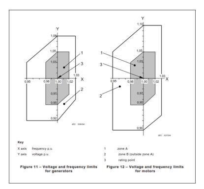
Figure 3: Voltage and frequency limits for generators and motors in BS EN 60034-1
