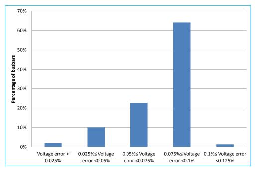
Figure 23 – Validation Results after PSS/E to IPSA Conversion
