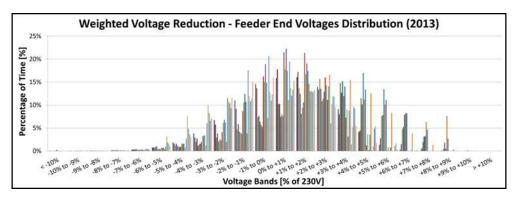
Figure 7: Distribution of feeder end voltages following a weighted voltage reduction of each 10 minute average measurement (y axis is the percentage of the year 2013)
