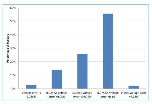
Figure 24 – Validation Results after Network Reduction
