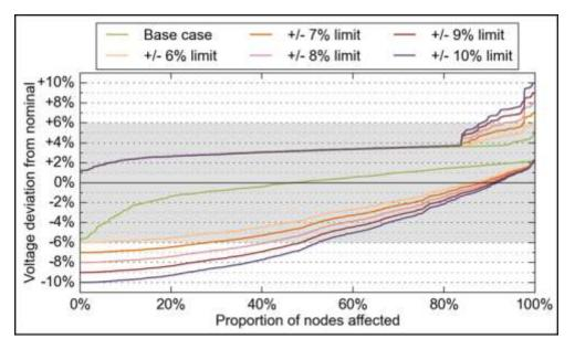
Figure 10: Cumulative frequency plots of steady state voltages for the high and low voltage cases when widened voltage limits applied at 11kV (results from the downstream models)
