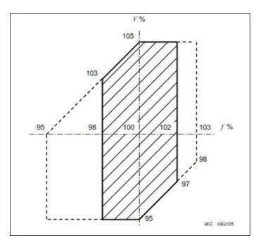
Figure 4: Operation over ranges of voltage and frequency is BSEN 60043-3
