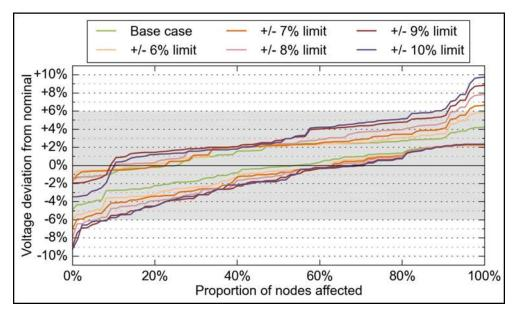
Figure 8: Cumulative frequency plots of steady state voltages for the high and low voltage cases when widened voltage limits are applied at 33kV (results from upstream model)
