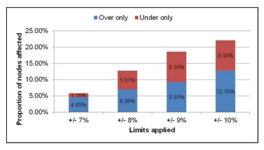
Figure 9: Proportion of 33kV nodes outside the current statutory limits
