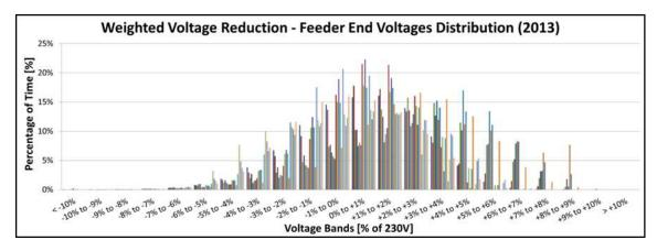
Figure 12: Distribution of feeder end voltages following a weighted voltage reduction
