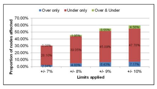
Figure 11: Proportion of 11kV nodes outside the current statutory limits
