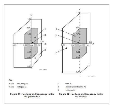
Figure 3: Voltage and frequency limits for generators and motors in BS EN 60037-1
