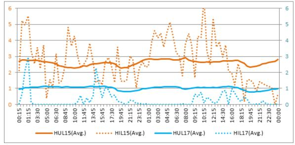
Figure 11: 5<sup>th</sup> & 7<sup>th</sup> Voltage and Current harmonics
