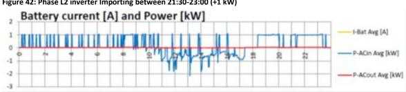
Figure 42: Phase L2 inverter Importing between 21:30-23:00 (+1 kW)
