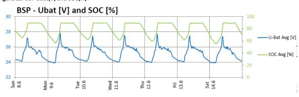
Figure 23: BSP Ubat(V) and SOC(%)
