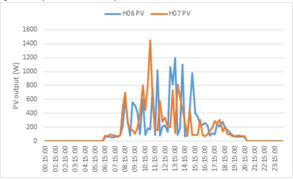
Figure 30: PV output of House 6 and 7 on 16 April
