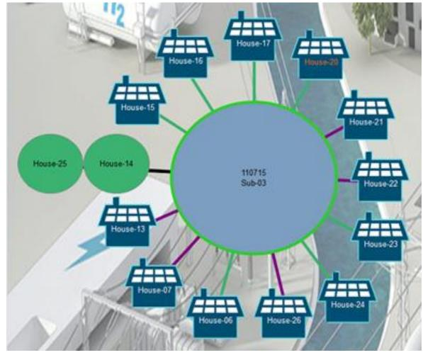
Figure 53: HMI display of the LV substation chosen for domestic property network trials & its connected properties
