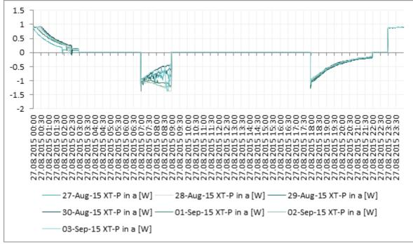
Figure 35: Power being exported to the grid in kW during AM and PM
