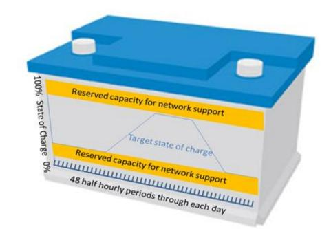
Figure 3: graphical representation of the EMS operation
