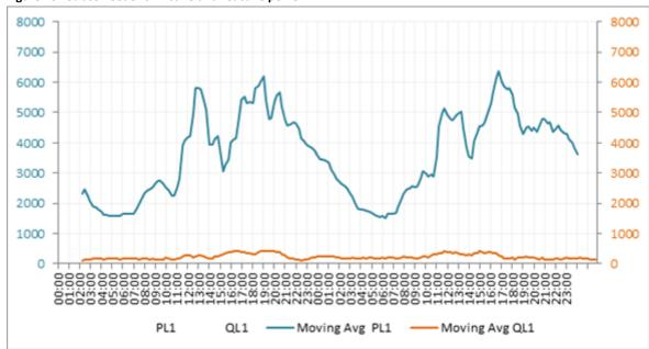
Figure 10: Sub05 Feeder 02 Active and reactive power
