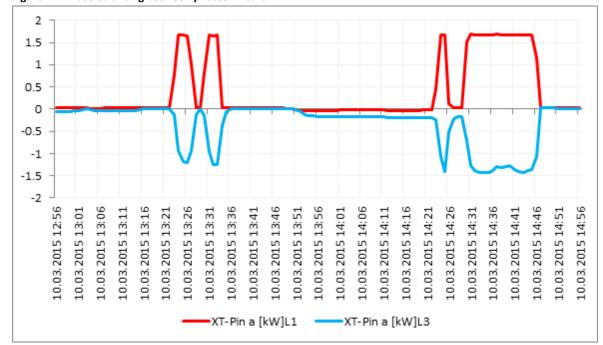
Figure 44: Phase balancing between phases L1 & L3
