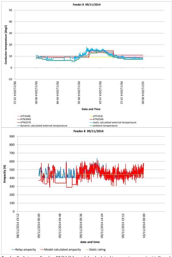
Feeder 8 : Autumn Sunday 08/11/14, model calculated temperature against toll grade reported temperature, model calculated ampacity against relay calculated ampacity
