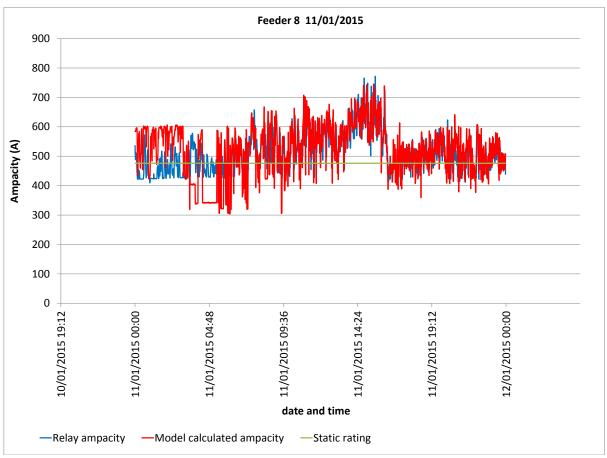
Feeder 8 : Winter Sunday 11/01/15, model calculated temperature against toll grade reported temperature, model calculated ampacity against relay calculated ampacity
