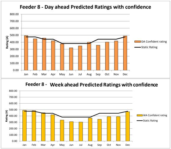
Figure 32 : 90% confidence calculated Ampacity Benefits using a) day ahead predicted data (75A) and b) week ahead predicted data (100A) for Feeder 8 over the course of a year with a 90% confidence level
