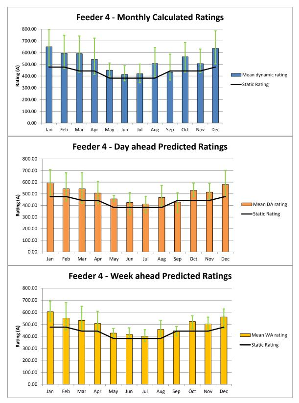
Figure 29 : Calculated Ampacity Benefits using a) measured data b) day ahead predicted data and c) week ahead predicted data for Feeder 4 over the course of a year
