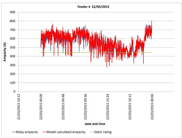
Feeder 4 : Spring Sunday 22/03/15, model calculated temperature against toll grade reported temperature, model calculated ampacity against relay calculated ampacity
