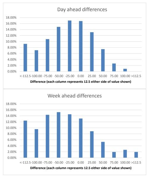
Figure 35 : Ampacity Error frequency plot on feeder 9for a) day ahead predicted data vs measured data b) week ahead predicted data vs measured data
