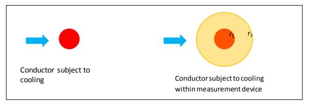
Figure 15 : Line temperature measurement device effect on cooling
