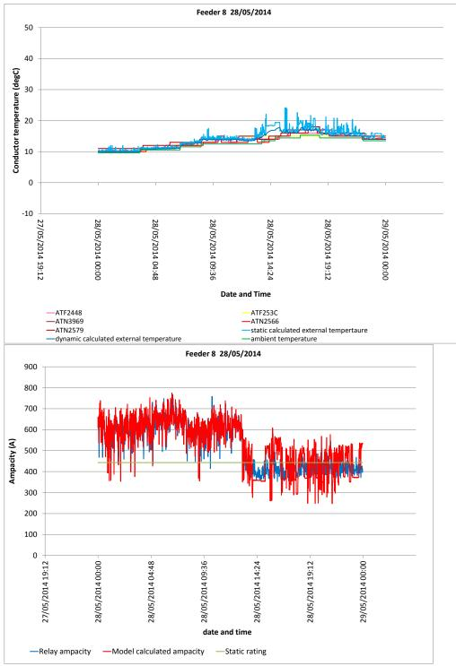
Feeder 8 :Spring Wednesday 28/05/15, model calculated temperature against toll grade reported temperature, model calculated ampacity against relay calculated ampacity
