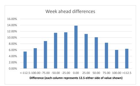
Figure 31 : Ampacity Error frequency plot on feeder 8 for a) day ahead predicted data vs measured data b) week ahead predicted data vs measured data
