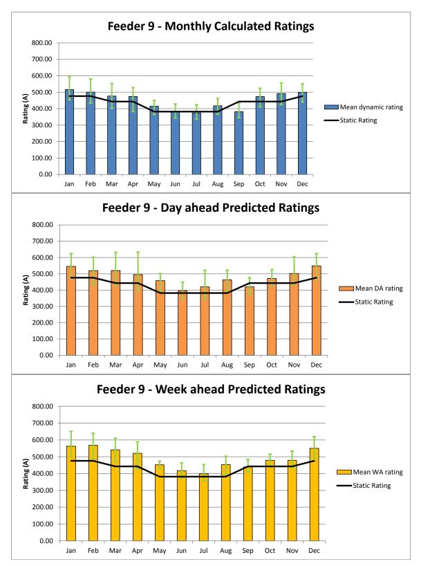
Figure 30 : Calculated Ampacity Benefits using a) measured data b) day ahead predicted data and c) week ahead predicted data for Feeder 9 over the course of a year
