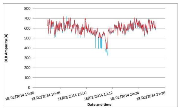
Figure 17 : DLR Ampacity against time (relay reported ampacity (red) and adjusted model values (blue))
