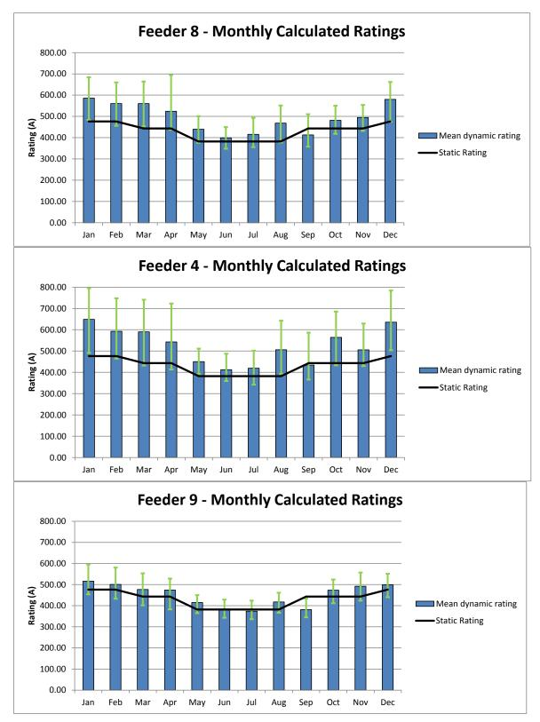
Figure 24 : Calculated Ampacity Benefits using measured data Feeders 8, 4 and 9 over the course of a year
