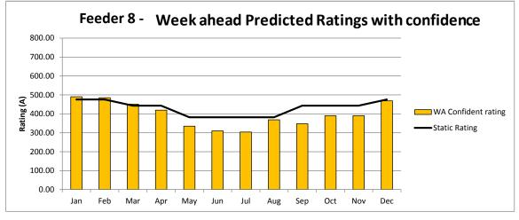
Figure 25 : Calculated Ampacity Benefits using a) measured data b) day ahead predicted data with 90% confidence and c) week ahead predicted data with 90% confidence over the course of a year
