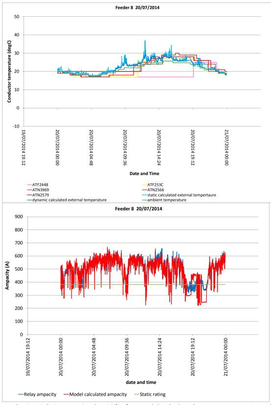
Feeder 8 : High Summer Sunday 20/07/14, model calculated temperature against toll grade reported temperature, model calculated ampacity against relay calculated ampacity
