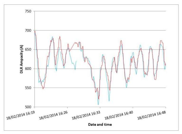
Figure 18 : Close-up of DLR Ampacity against time (relay reported ampacity (red) and adjusted model values (blue))
