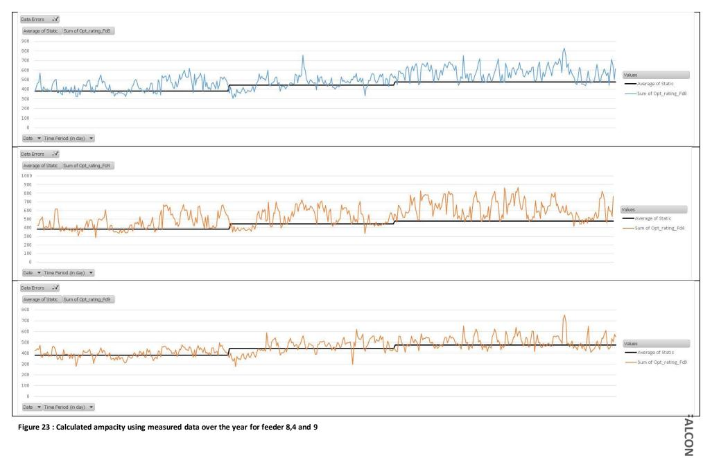
Figure 23 : Calculated ampacity using measured data over the year for feeder 8,4 and 9
