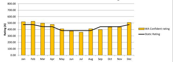
Figure 36 : 90% confidence calculated Ampacity Benefits using a) day ahead predicted data (40A) and b) week ahead predicted data (40A) for Feeder 9 over the course of a year with a 90% confidence level
