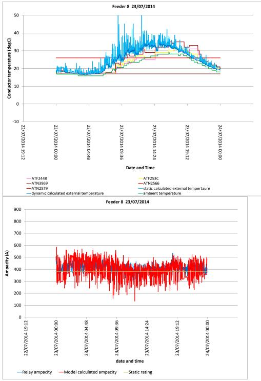
Feeder 8 : High Summer Wednesday 23/07/14, model calculated temperature against toll grade reported temperature, model calculated ampacity against relay calculated ampacity
