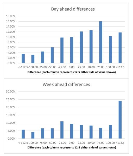
Figure 33 : Ampacity Error frequency plot on feeder 4 for a) day ahead predicted data vs measured data b) week ahead predicted data vs measured data
