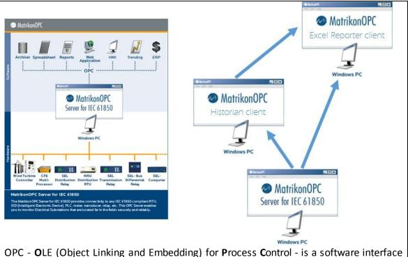
OPC - **O**LE (Object Linking and Embedding) for **P**rocess **C**ontrol - is a software interface standard that allows Windows programs to communicate with industrial hardware devices
