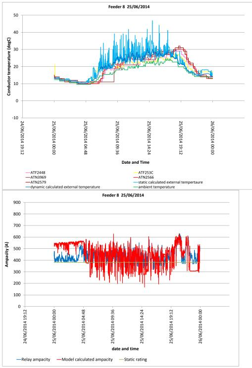
Feeder 8 : Summer Wednesday 25/06/14, model calculated temperature against toll grade reported temperature, model calculated ampacity against relay calculated ampacity
