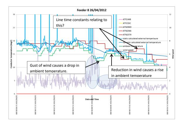
Figure 14 : Line temperature with changes in wind speed
