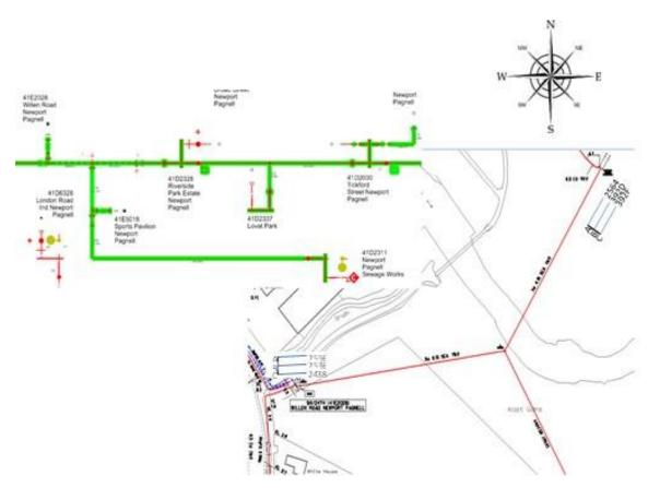
Figure 4: Feeder 4 Tollgrade sensor locations
