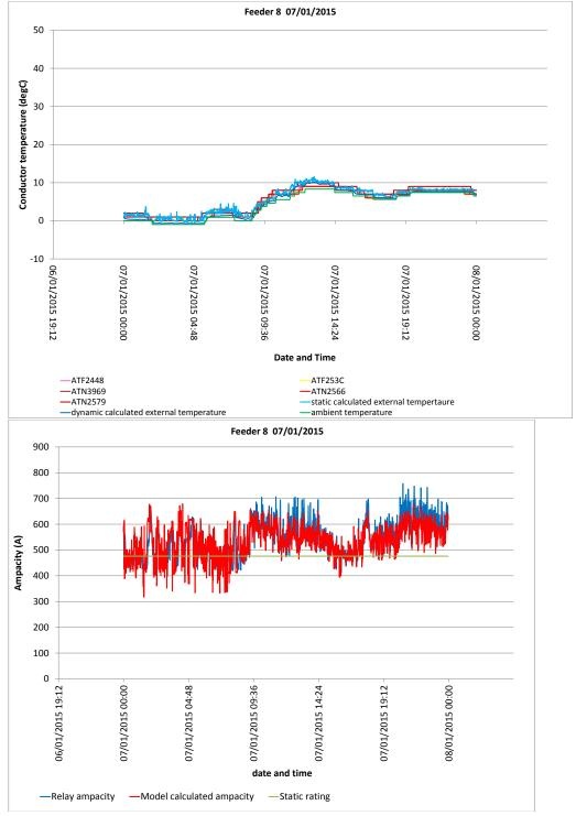
Feeder 8 : Winter Wednesday 07/01/15, model calculated temperature against toll grade reported temperature, model calculated ampacity against relay calculated ampacity
