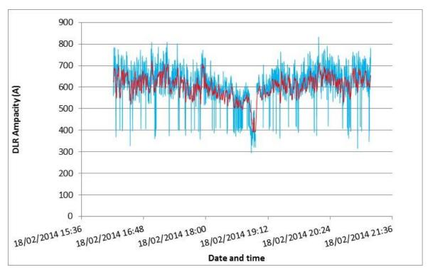
Figure 16 :DLR Ampacity against time (relay reported ampacity (red) and unmodified model values (blue))
