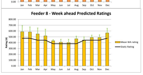
Figure 28 : Calculated Ampacity Benefits using a) measured data b) day ahead predicted data and c) week ahead predicted data for Feeder 8 over the course of a year
