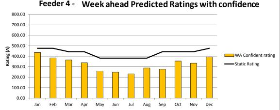
Figure 34 : 90% confidence calculated Ampacity Benefits using a) day ahead predicted data (120A) and b) week ahead predicted data (170A) for Feeder 4 over the course of a year with a 90% confidence level
