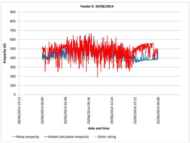
Feeder 8 : Summer Sunday 29/06/14, model calculated temperature against toll grade reported temperature, model calculated ampacity against relay calculated ampacity
