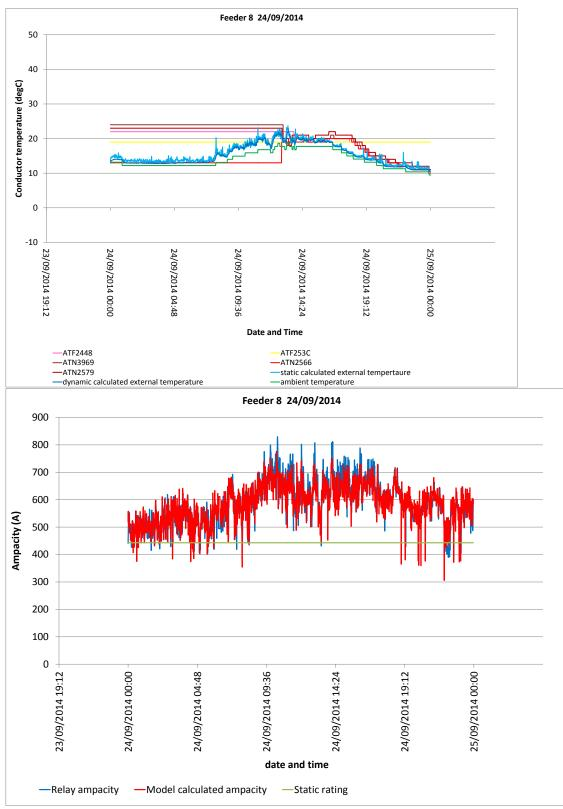
Feeder 8 : Autumn Wednesday 24/09/14, model calculated temperature against toll grade reported temperature, model calculated ampacity against relay calculated ampacity
