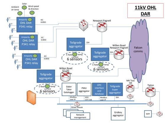
Figure 2: Schematic of installed 11kV OHL DAR scheme In summary, the installed equipment comprises of:
