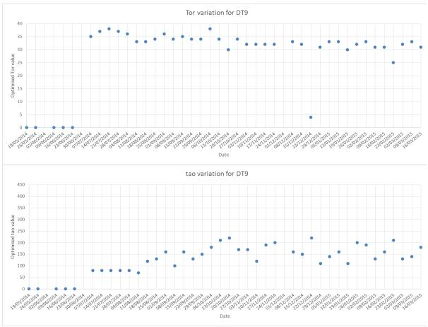
Tuned  $\Delta T_{tor}$  and  $\tau_o$  parameters for transformer 9
