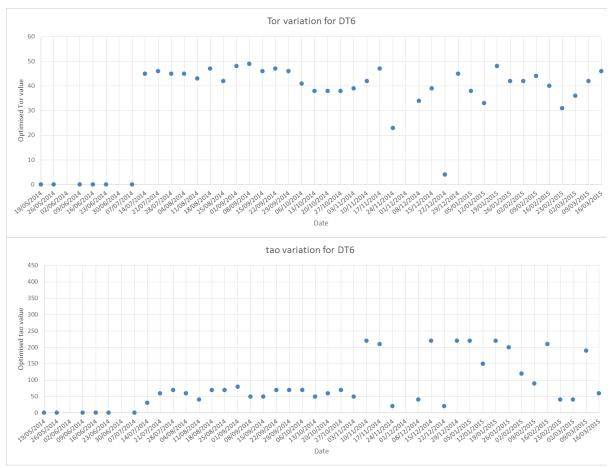
Tuned  $\Delta T_{tor}~$  and  $au_o$  parameters for transformer 6
