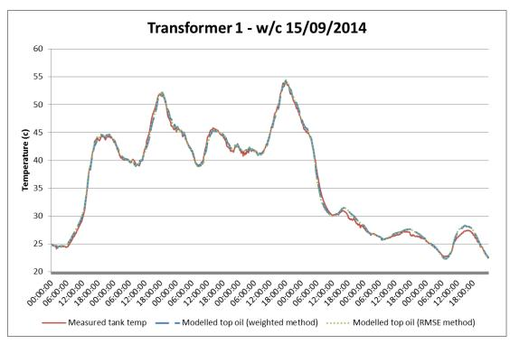
Figure 14 : Thermal model curves for transformer that can be reliably modelled
