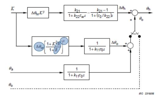
Figure 9 : IEC60076 showing constants that affect the value of calculated top oil temperature rise
