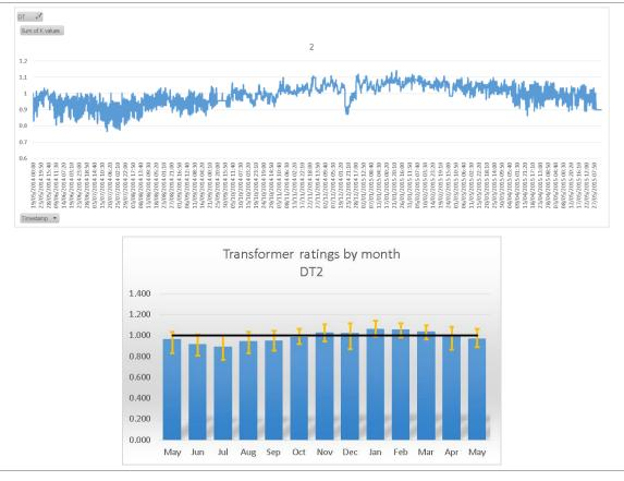
Figure 19: Calculated Dynamic asset rating at Granvills Square Distribution Transformer over the year and on a month by month basis.
