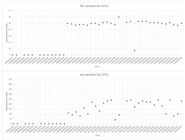
Tuned  $\Delta T_{tor}$  and  $\tau_o$  parameters for transformer 15
