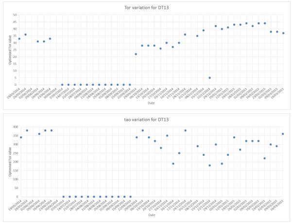
Tuned  $\Delta T_{tor}$  and  $\tau_o$  parameters for transformer 13
