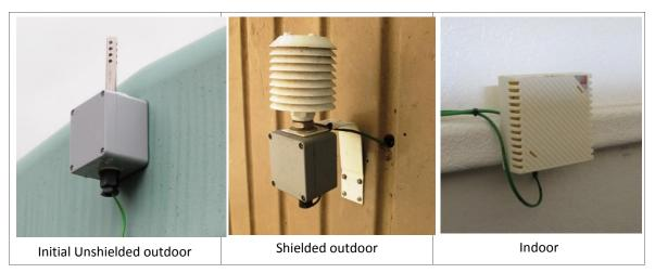
Figure 4 : Illustration of air temperature sensors, and positioning
