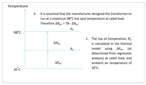
Figure 16 : Illustration of method for determining  $\Delta T_{hsr}$
