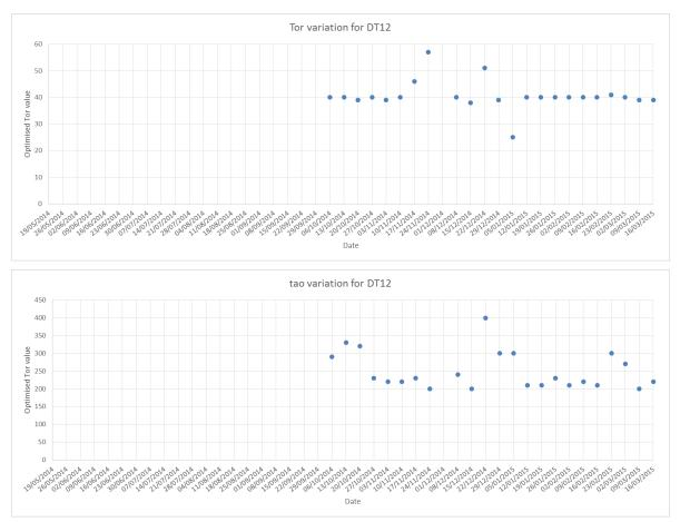
Tuned  $\Delta T_{tor}~$  and  $\tau_o$  parameters for transformer 12
