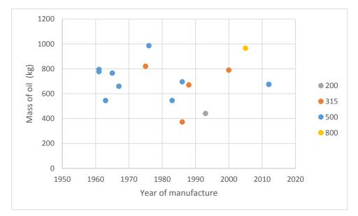
Figure 12 : Variation in mass of oil in transformers
