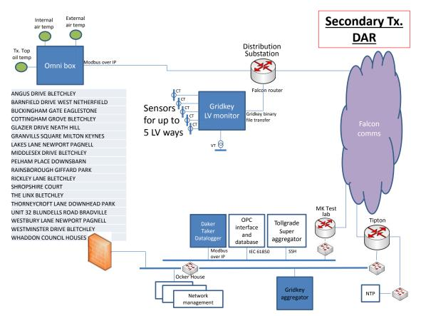
Figure 3 : Schematic of installed Distribution transformer DAR scheme
