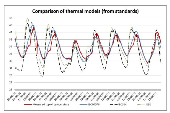
Figure 13 : Sample results of top oil temperature modelling via the three Industry Standards, and the measured oil temperature.
