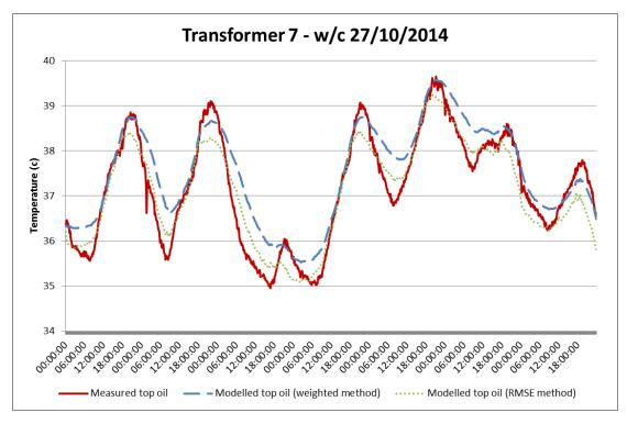
Figure 15 : Thermal model curves for transformer difficult to model
