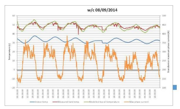
Figure 17: Correlation between calculated and measured top oil temperature for Rickley Lane
