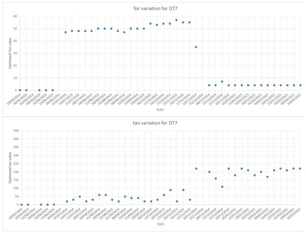
Tuned  $\Delta T_{tor}$  and  $\tau_o$  parameters for transformer 7
