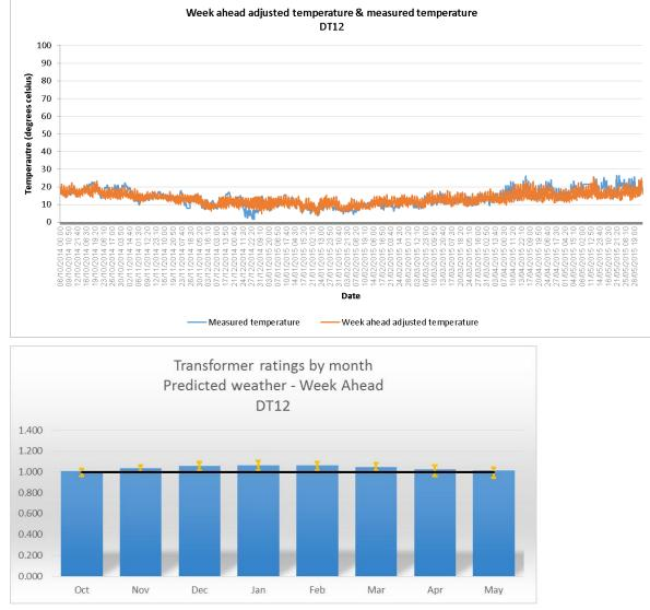
Transformer 12 : Predicted ambient temperature and predicted benefits (data for Transformer 12 only valid from Oct 2014 onwards)
