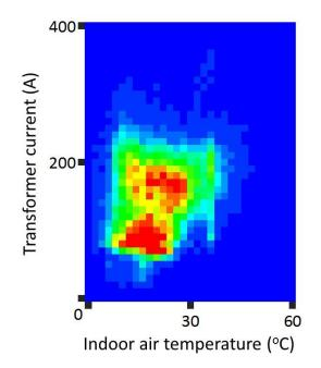
Figure 18: Heat map-style representation of range of load and ambient air temperatures experienced at Granvills Square Distribution Transformer.
