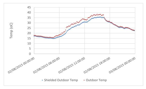
Figure 5 : Difference in measured air temperature with and without a Stevenson Shield – The Linx, Bletchley
