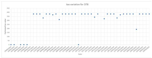
Tuned  $\Delta T_{tor}$  parameters for transformer 8
