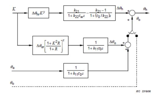
A number of model parameters (e.g. ΔΘ<sub>or</sub>, R, x etc.) that are used within the calculation.
