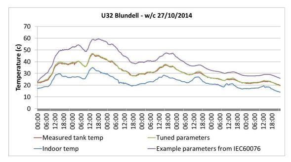
example set of values results in an overestimation of top oil temperature of up to  $15^{\circ}$ C compared to measured values.
