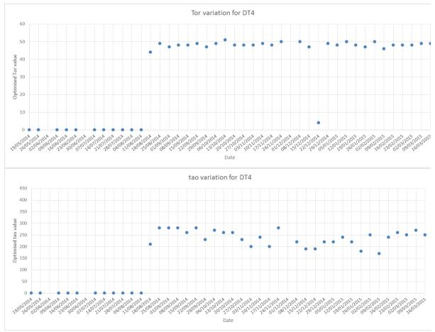
Tuned  $\Delta T_{tor}$  and  $au_o$  parameters for transformer 4
