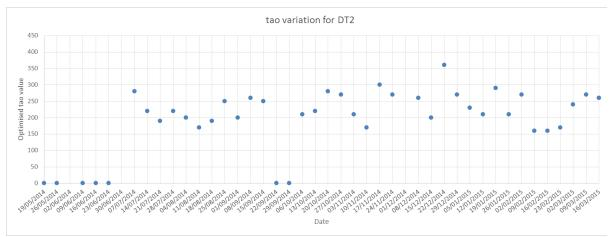
Tuned  $\Delta T_{tor}$  and  $\tau_o$  parameters for transformer 2
