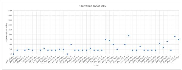
Tuned  $\Delta T_{tor}$  and  $au_o$  parameters for transformer 5
