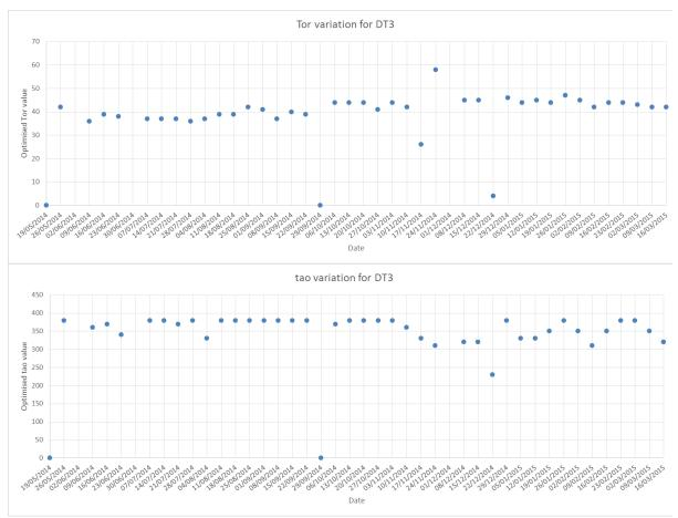
Tuned  $\Delta T_{tor}~$  and  $au_o$  parameters for transformer 3
