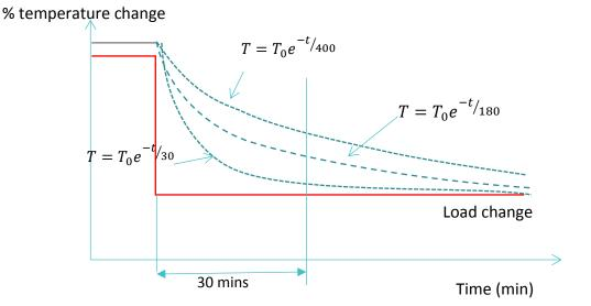
Figure 11 : effect of time constant on accuracy of temperature calculation
