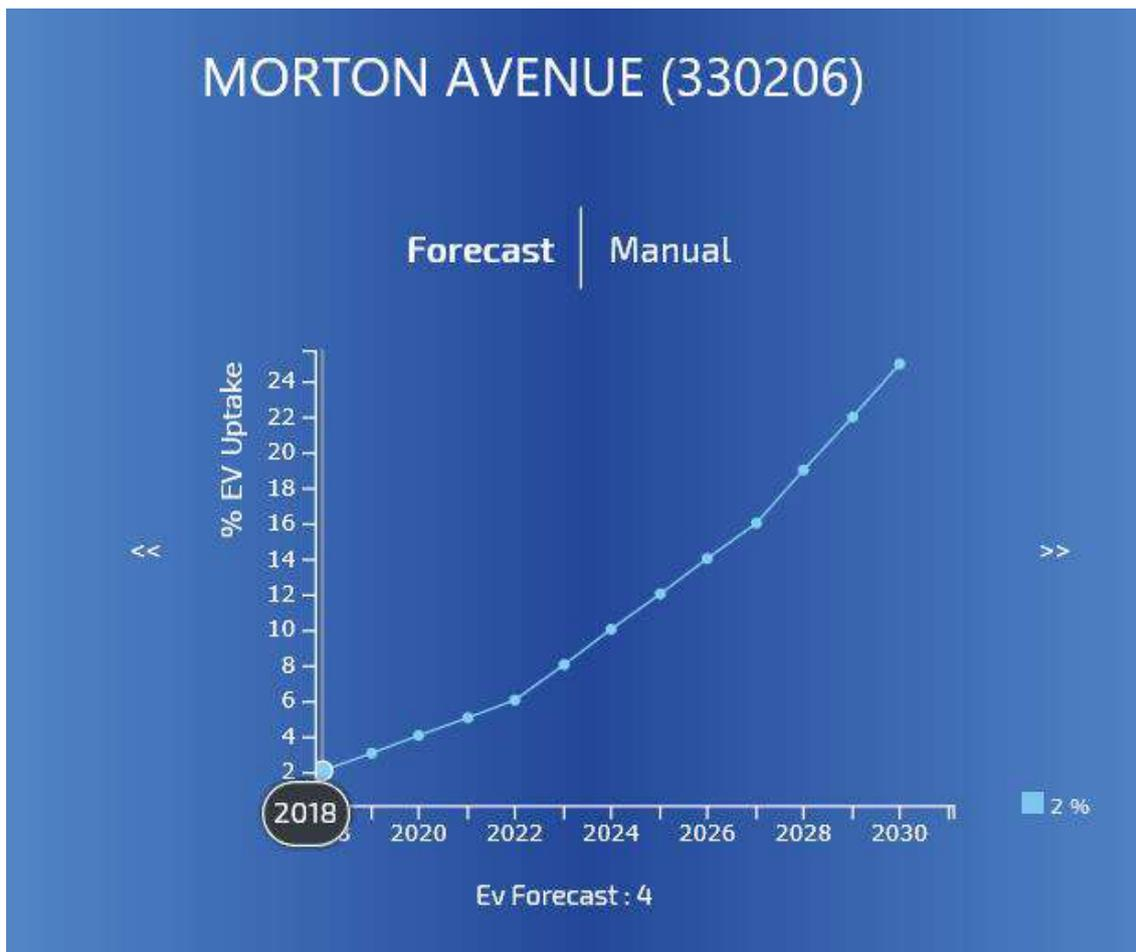
Figure 8: The forecasting functionality in operation. This shows the predicted number of EVs using the network associated with the selected LV substation on a given year. Note the modified legend showing the number of EVs on the network and the percentage EV penetration.
