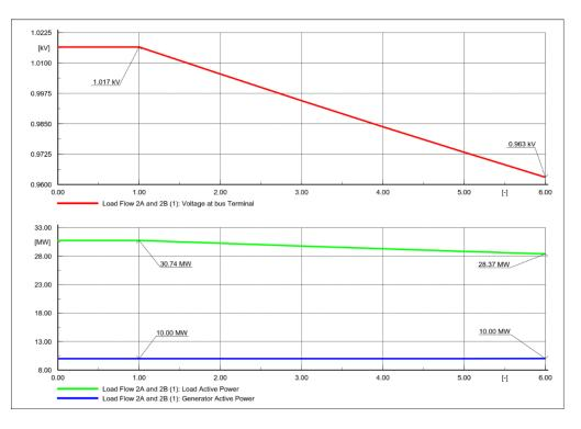
Figure 6-15 – Transformer tap changed from -4 to 1 by CLASS with no ANM reaction
