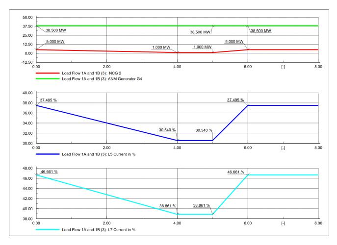
Figure 6-6 - Non-curtailable generator 2 decrement and all cables in service
