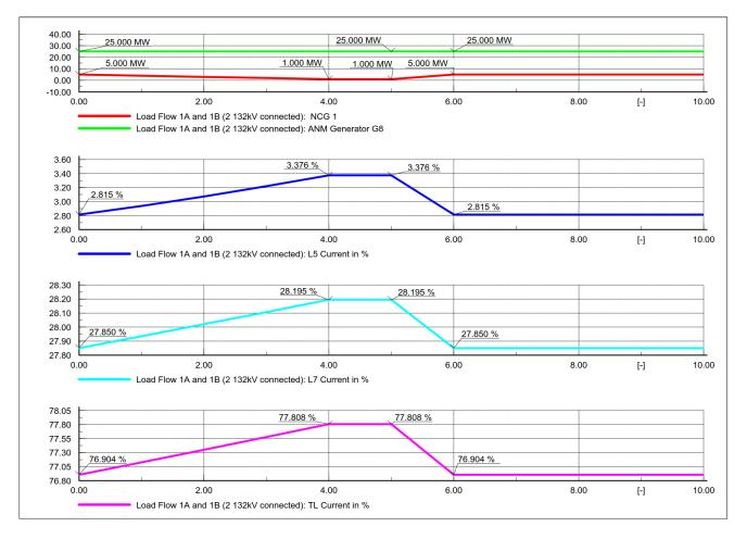
Figure 6-10 - W1: Non-curtailable generator 1 decriment and L1 out of service
