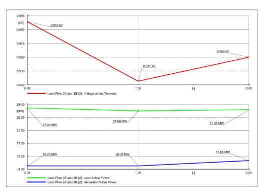
Figure 6-18 - Transformer (T6) taken out of service, initial tap position of 2 with ANM reaction
