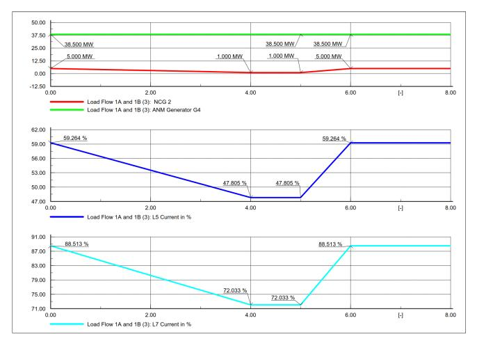
Figure 6-8 - W1: Non-curtailable generator 2 decrement and L6 out of service
