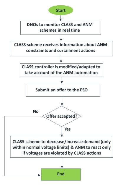
Figure 5-5 - Z2 solution flow chart
