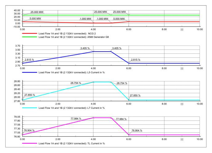
Figure 6-13 - W1: Non-curtailable generator 2 decriment and L1 out of service
