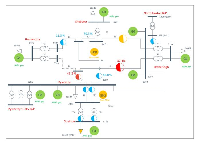
Figure 6-2 – Schematic layout of the test network model with additional 132kV connection
