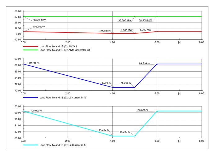
Figure 6-7 - W1: Non-curtailable generator 2 decrement and L1 out of service
