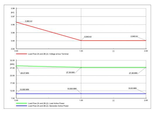
Figure 6-17 – Transformer (T6) taken out of service, initial tap position of 1 with no ANM reaction
