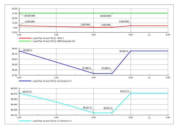
Figure 6-5 - W1: Non-curtailable generator 1 decrement and L6 out of service
