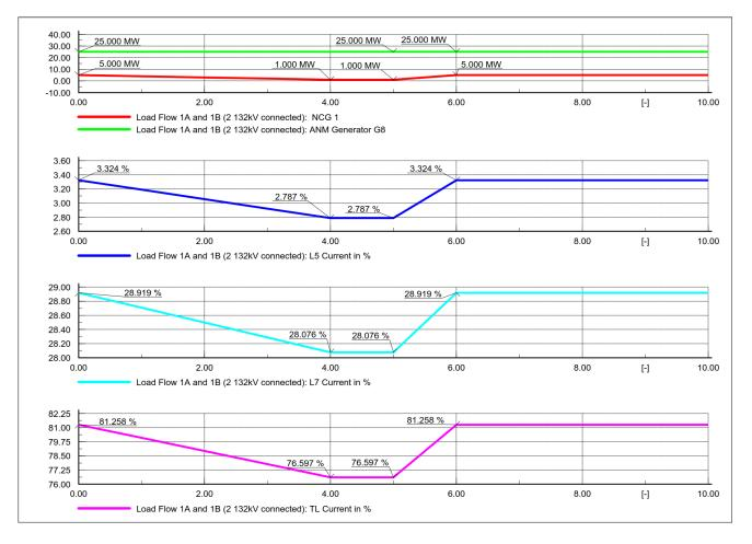
Figure 6-9 - W1: Non-curtailable generator 1 decriment and all cables in service
