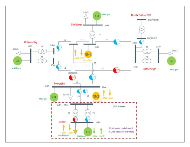
Figure 6-1 – Schematic layout of the test network model
