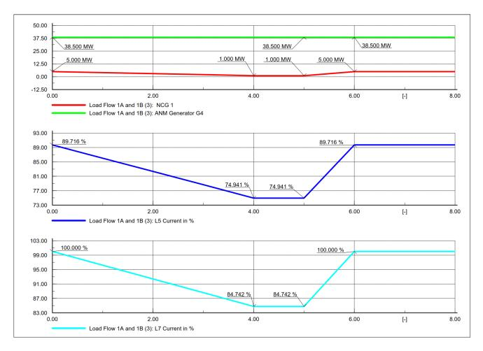
Figure 6-4 - W1: Non-curtailable generator 1 decrement and L1 out of service
