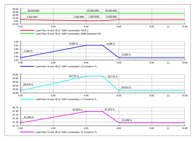
Figure 6-12 - W1: Non-curtailable generator 2 decriment and all cables in service
