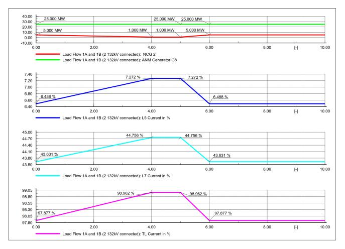
Figure 6-14 - W1: Non-curtailable generator 2 decriment and L6 out of service
