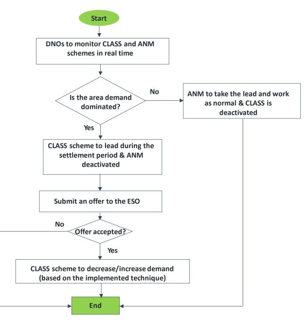
Figure 5-4 - Z1 solution flow chart
