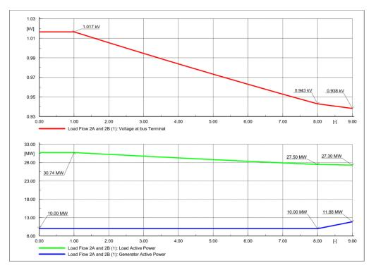
Figure 6-16 - Transformer tap changed from - 4 to 4 by CLASS vs ANM reaction
