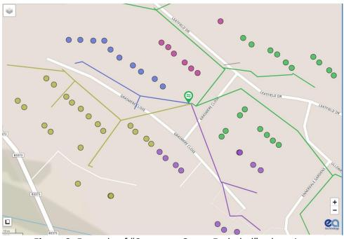
Figure 3: Example of "Customer Group Excluded" substation.
