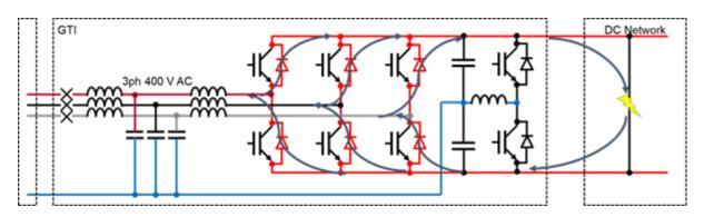
Figure 2: Fault current path in the GTI
