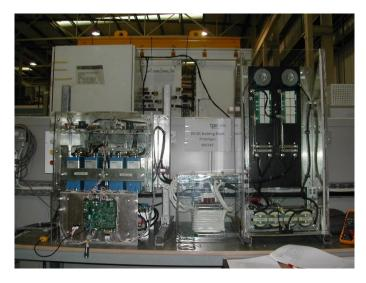
Figure 18: Resonant DC-DC Converter 2020 (utilising FUN-LV GTI)
