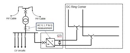
Figure 19: GTI Interfacing
