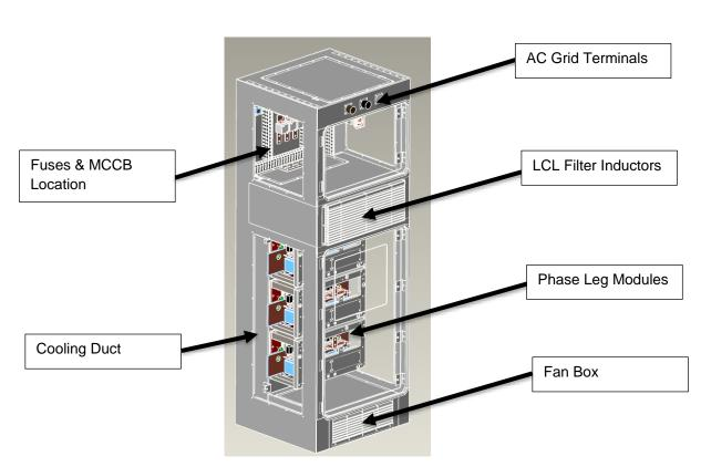
Figure 6 Inverter Enclosure Internal View
