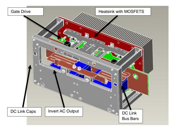
The inverter leg heat sink can cool three MOSFET modules (CREE CAS300M12BM2) connected in parallel. When three modules are formed into a 3-phase inverter it is capable of handling 400kVA.
