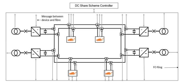
Figure 8. Schematic Representation of the DC Share Solution
