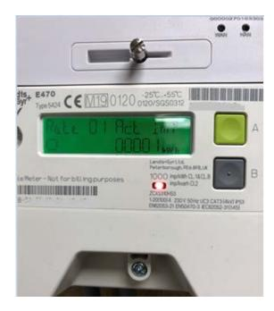
The main screen on the meter is already defaulted to the Import Register which shows your reading. Please use this when submitting your meter reading.
