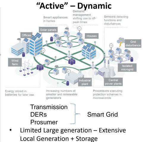
Focus on balancing demand and availability through the the transition to embedded generation and alternative gases
